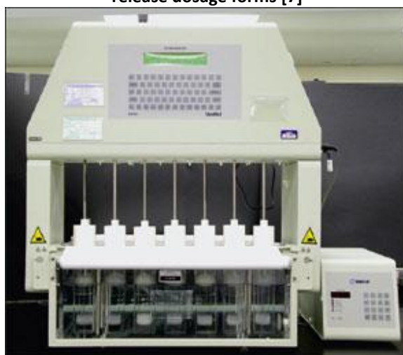
Figure 3: The advantages of USP Apparatus 3 include ease of setup, operation, and sampling. It is generally preferred when a pH gradient is required [7].
