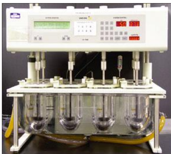
Figure 2: Dissolution Apparatus 1 and 2 is generally the first choice for measuring the dissolution of immediate release dosage forms [7]
