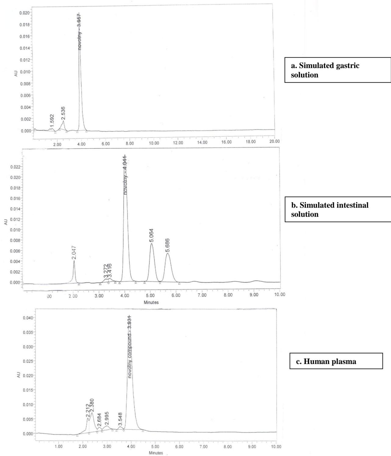
**Fig. 2. HPLC chromatograms of P763 in simulated gastric solution (a), simulated intestinal solution (b) and human plasma (c) at 37°C ±1 after incubation for 5 hours**
