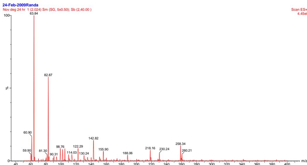
Fig. 5. MS scan of the degraded solution of P763 after incubation in phosphate buffer solution, pH 7.4 at 37°C±1 for 24 hours.
