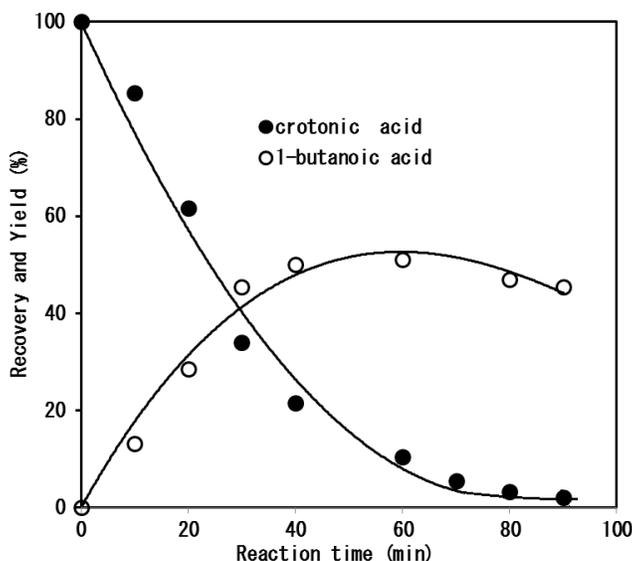
**Fig. 8:** Formation of 1-butanoic acid from an aqueous solution of crotonic acid (10 mM) at 30 °C induced by argon–hydrogen plasma jet blowing at the gas flow rates: argon 1.5 L/min and hydrogen 0.5 L/min. Electric current and voltage were maintained at 30 A and 15 V, respectively. ●: crotonic acid, ○: 1-butanoic acid.
