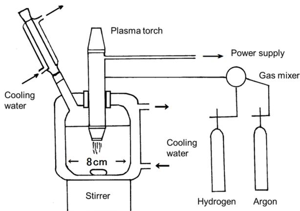
**Fig 1: Apparatus for argon–hydrogen plasma jet blowing.**
