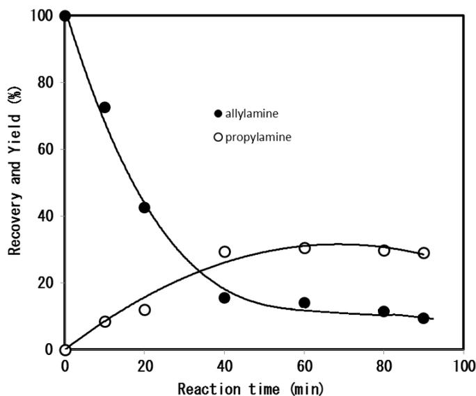
**Fig. 10:** Formation of propylamine from an aqueous solution of allylamine (10 mM) at 30 °C induced by argon–hydrogen plasma jet blowing at the gas flow rates: argon, 1.5 L/min and hydrogen, 0.5 L/min. Electric current and voltage were maintained at 30 A and 15 V, respectively. ●: allylamine, ○: propylamine.
