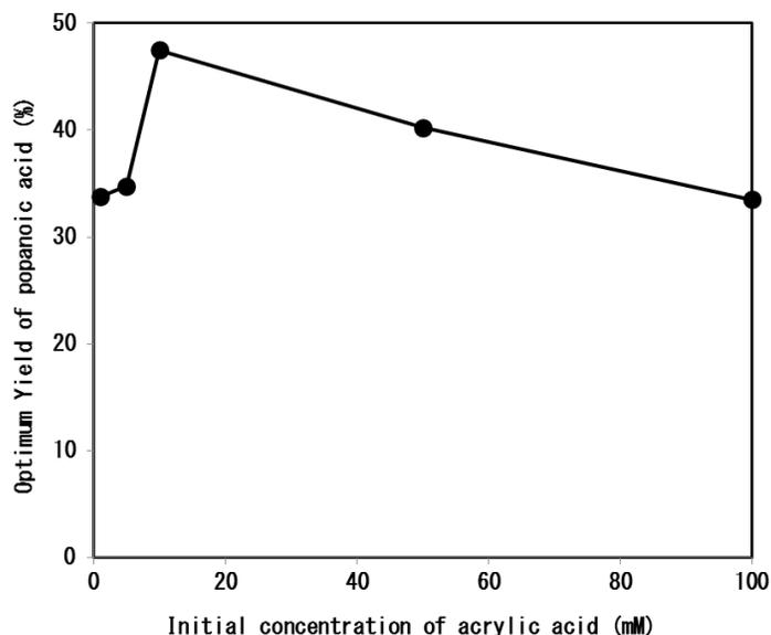
**Fig. 4:** Correlation between the initial concentration of acrylic acid and the optimum yield of propanoic acid at 30 °C induced by argon–hydrogen plasma jet blowing at the gas flow rates: argon 1.5 L/min and hydrogen 0.5 L/min. Electric current and voltage were maintained at 30 A and 15 V, respectively.
