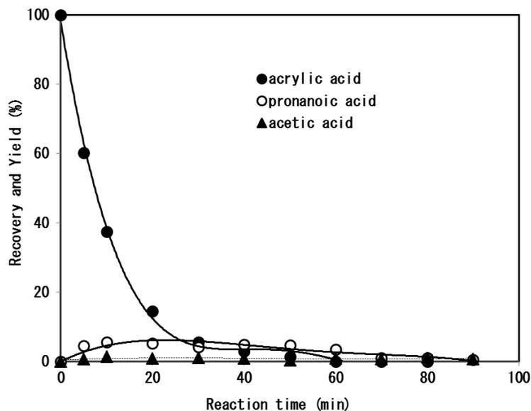
Fig. 6: Formation of propanoic acid from an aqueous solution of acrylic acid (10mM) at 30 °C induced by argon-hydrogen plasma jet blowing at the gas flow rates: argon 2.0 L/min and hydrogen 0.0 L/min. Electric current and voltage were maintained at 30 A and 15 V, respectively. ●: acrylic acid, ○: propanoic acid, ▲: acetic acid.
