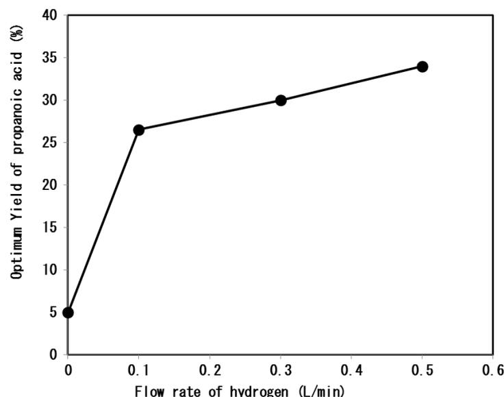
**Fig. 3:** Correlation between the flow rate of hydrogen and the optimum yield of propionic acid from an aqueous solution of acrylic acid (0.1 M) at 30 °C induced by argon–hydrogen plasma jet blowing at the gas flow rates: argon 1.5 L/min and hydrogen 0.5 L/min. Electric current and voltage were maintained at 30 A and 15 V.
