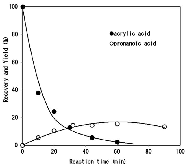
**Fig. 7:** Formation of propanoic acid from acrylic acid (10 mM) in 10% formic acid at 30 °C induced by argon-hydrogen plasma jet blowing at the gas flow rates: argon 2.0 L/min. Electric current and voltage were maintained at 30 A and 15 V, respectively. ●: acrylic acid, ○ propanoic acid.
