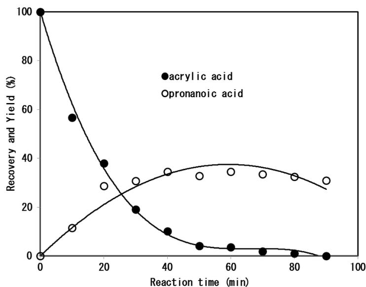
**Fig 2: Formation of propanoic acid from an aqueous solution of acrylic acid (100mM) at 30 °C induced by argon–hydrogen plasma jet blowing at the gas flow rates: argon 1.5 L/min and hydrogen 0.5 L/min. Electric current and voltage were maintained at 30 A and 15 V, respectively. ●: acrylic acid, ○: propanoic acid.**
