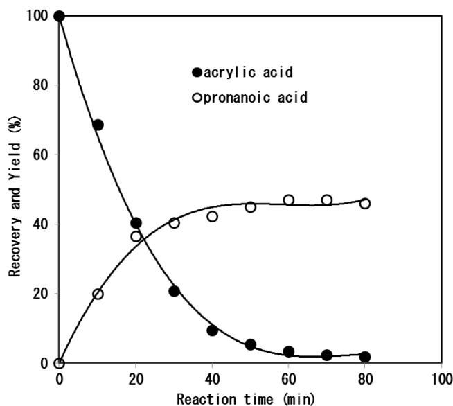
**Fig. 5:** Formation of propanoic acid from an aqueous solution of acrylic acid (10mM) at 30 °C induced by argon–hydrogen plasma jet blowing at the gas flow rates: argon 1.5 L/min and hydrogen 0.5 L/min. Electric current and voltage were maintained at 30 A and 15 V, respectively. ●: acrylic acid, ○:propanoic acid.
