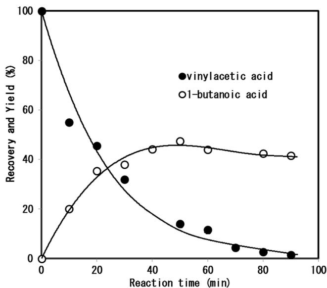
**Fig. 9:** Formation of 1-butanoic acid from an aqueous solution of vinylacetic acid (10 mM) at 30 °C induced by argon–hydrogen plasma jet blowing at the gas flow rates: argon 1.5 L/min and hydrogen 0.5 L/min. Electric current and voltage were maintained at 30 A and 15 V, respectively. ●: vinylacetic acid, ○: 1-butanoic acid.
