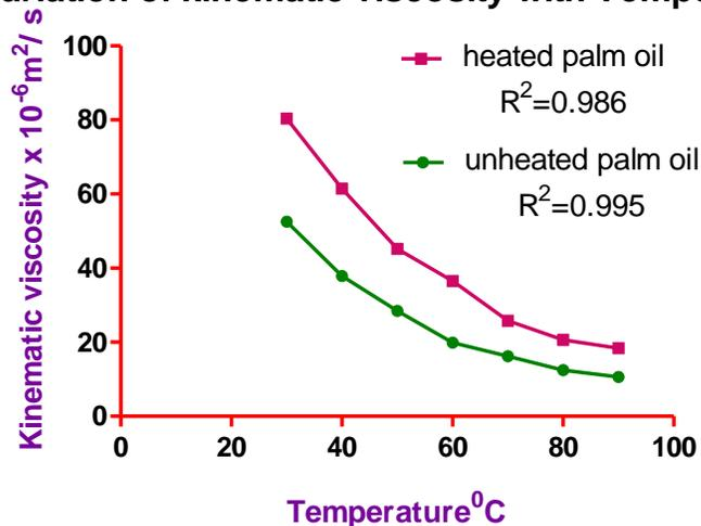
Figure 1: Variation of viscosity with temperature of palm oil
