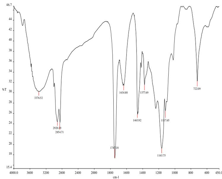
Figure 4 FTIR spectrum of heated Palm oil
