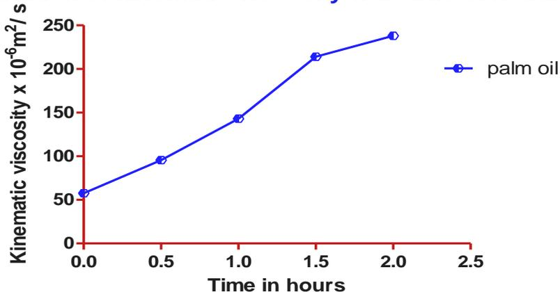
Figure 2: Variation of kinematic viscosity with time of heating
