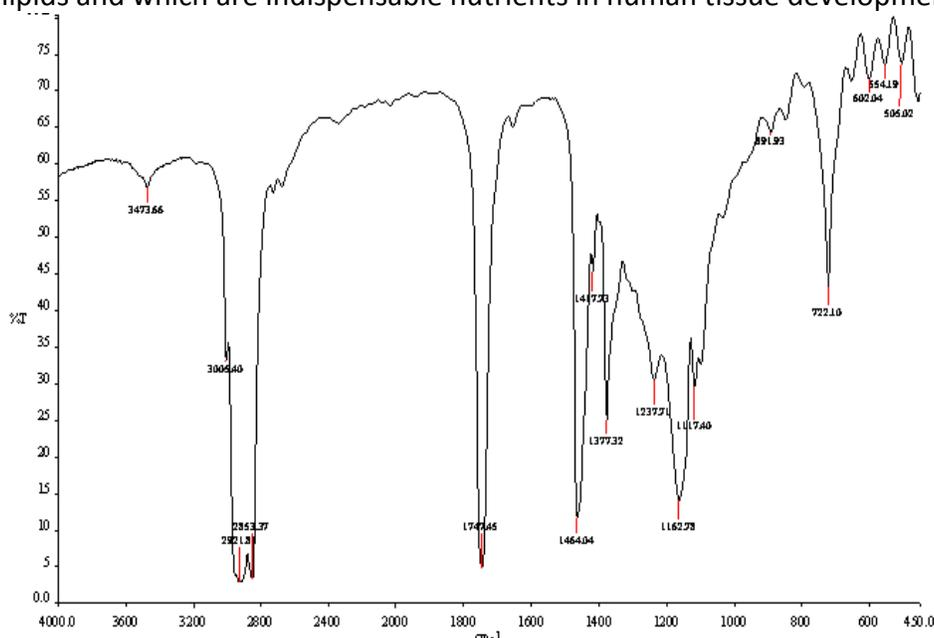
Figure 3 FTIR spectrum of unheated Palm oil
