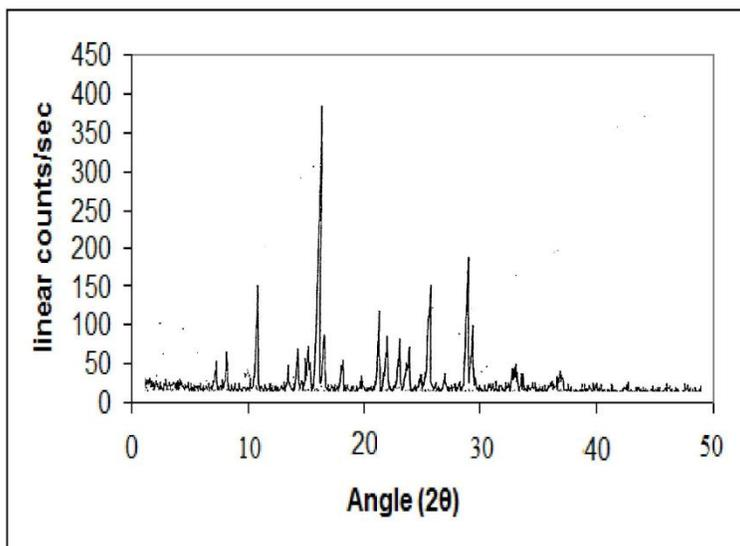
Fig 4: XRD spectra of Plasdone K12
