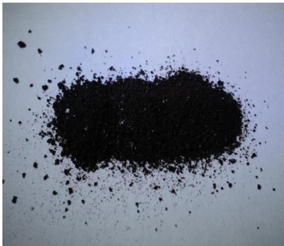
Fig.5: ZrO nanoparticles
