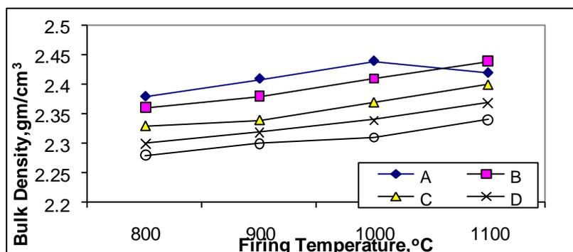
Figure (2) Effect of firing temperature from 800°C up to 1100°C on the bulk density of tested samples having 0-10% of cement dust
