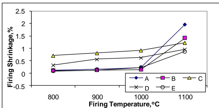
Figure (1) Effect of firing temperature from 800°C up to 1100°C on the shrinkage of tested samples having 0-10% of cement dust
