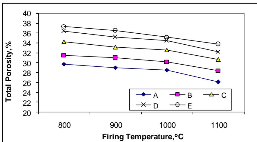
Figure (3) Effect of firing temperature from 800 °C up to 1100°C on the Total Porosity of tested samples having 0-10% of cement dust
