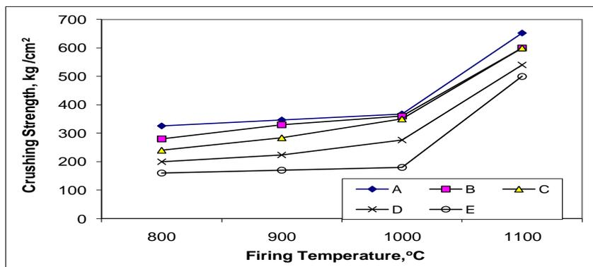
Figure (4) Effect of firing temperature from 800 °C up to 1100°C on the Crushing Strength of tested samples having 0-10% of cement dust
