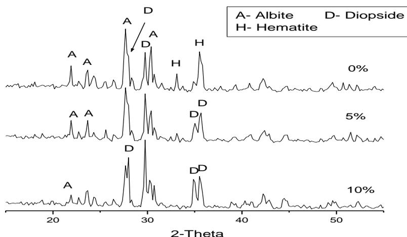
Figure (5): XRD patterns of the fired samples containing 0, 5, and 10% cement dust fired at 1100°C.
