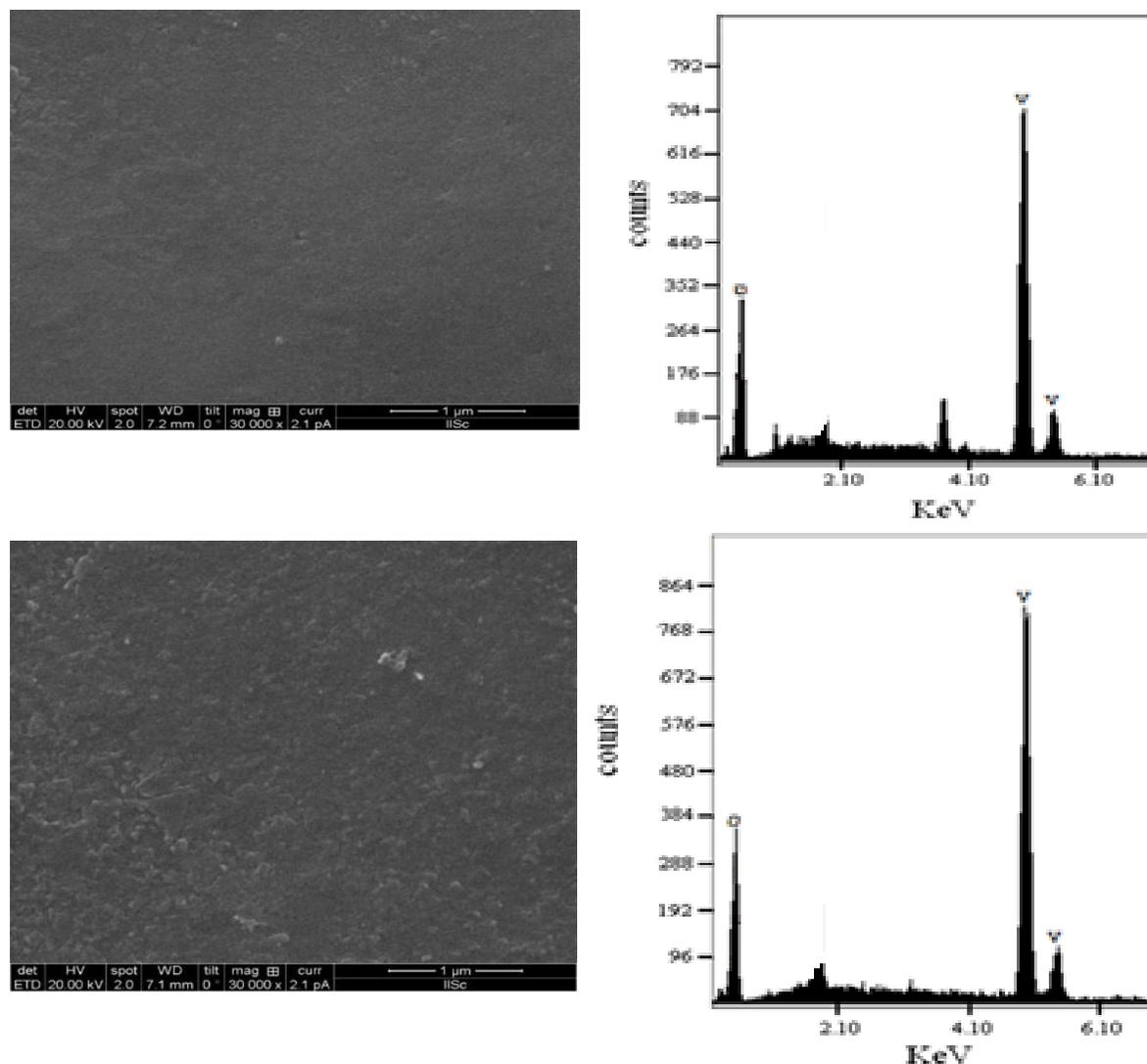
Fig 2 (a-c) SEM and EDAX pattern of  $V_2O_5$  thinfilms obtained at different temperatures
