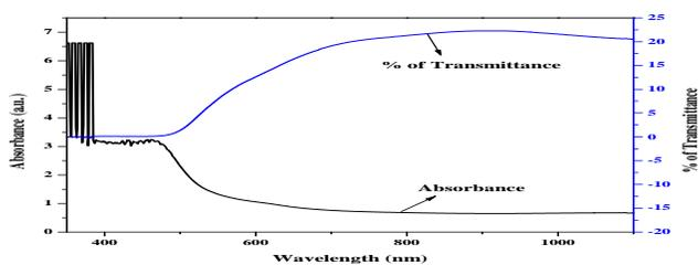
Figure 3 (a-c): UV – VIS Absorbance and Transmittance of V<sub>2</sub>O<sub>5</sub> thinfilms obtained at different temperatures
