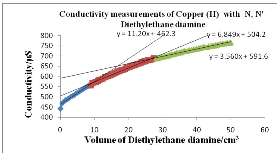
Figure 14: Conductivity measurements for N, N' Diethylethane
