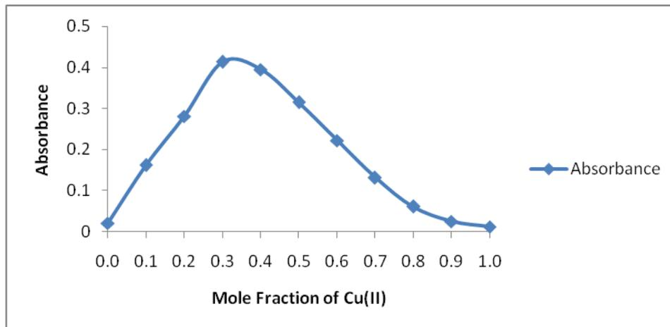
Figure 13: Job's Plot for Cu(II)-N,N'-Diethylethane diamine.
