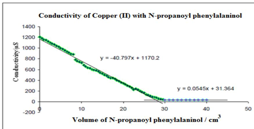
Figure 16: Conductivity measurements for N-propanoyl phenylalaninol
