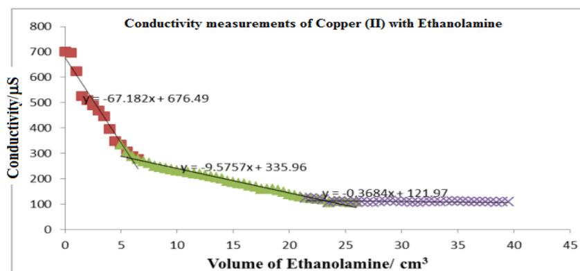
Figure 6: Conductivity measurements for ethanolamine
