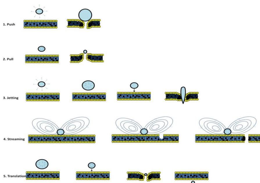
Figure 1: Mechanism of pore formation.
