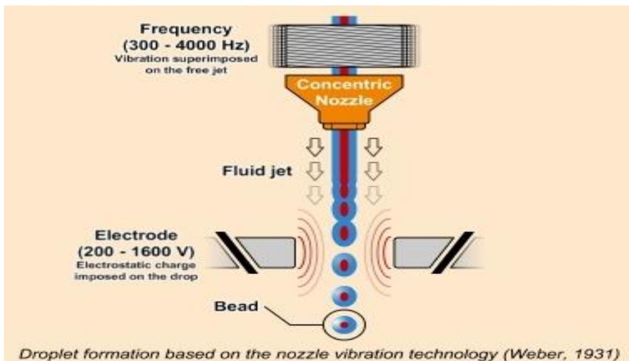
Fig 2: Droplet Formation Based On The Nozzle Vibration Technology
