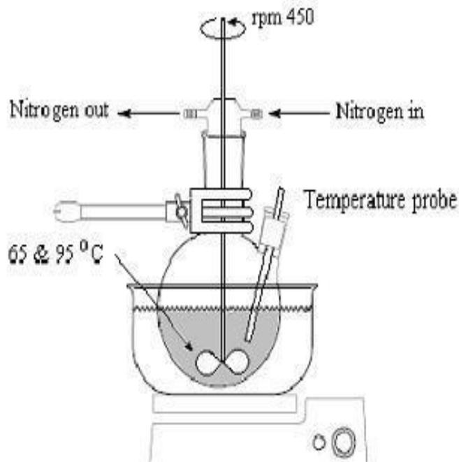
**Figure 2: Reaction vessel for microsphere preparation by liquid-liquid suspension polymerization [26]**
