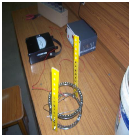
Figure 3c: Ring-power supply set up with an Ammeter and DC generator for preliminary studies on different solutions
