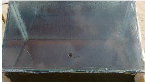
Figure 1: Design for solar reactor (5 liter human urine) as lab-scale
