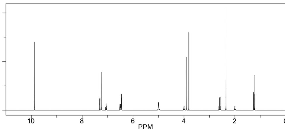
**Figure 3: <sup>1</sup>H NMR Spectra of 4 – HBPHF-II Copolymer resin**
