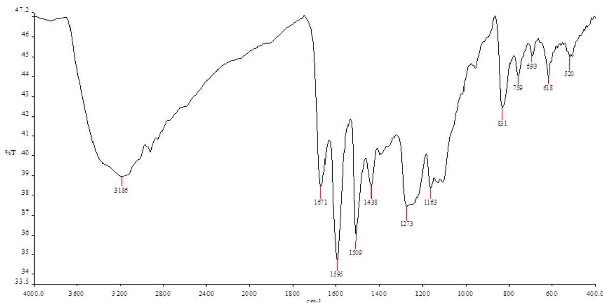
**Figure 2: Infra-Red Spectra of 4 – HBPHF-II Copolymer resin**
