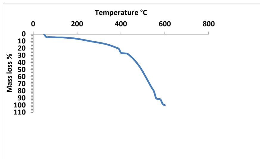
**Figure 4: Decomposition pattern of 4 – HBPHF-II Copolymer resin.**
