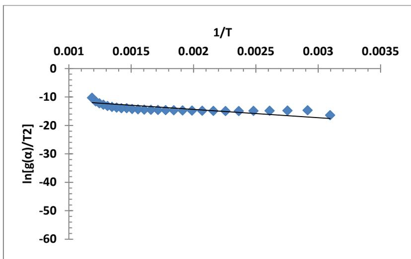
Figure 11: Coat Redfern plot plot of 4 – HBPHF-II Copolymer resin
