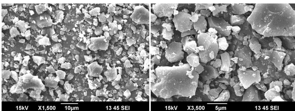
Figure 12: SEM photograph (a, b) of 4 – HBPHF-II Copolymer resin
