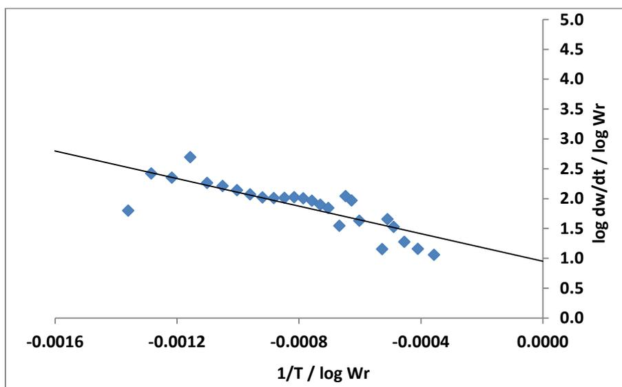
Figure 5: Freeman- Caroll plot 1 of 4 – HBPHF-II Copolymer resin for activation energy and order of reaction
