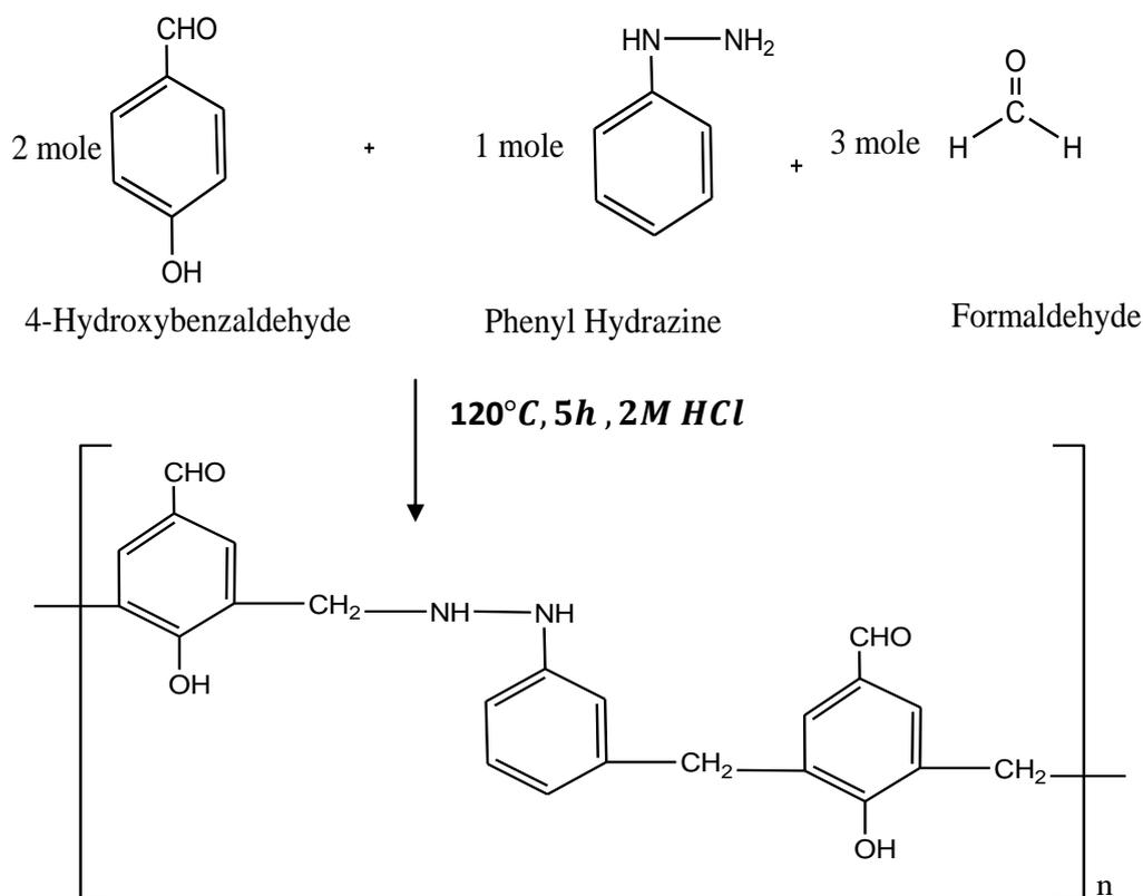
Figure 1: Reaction and suggested structure of 4 – HBPHF -II Copolymer resin
