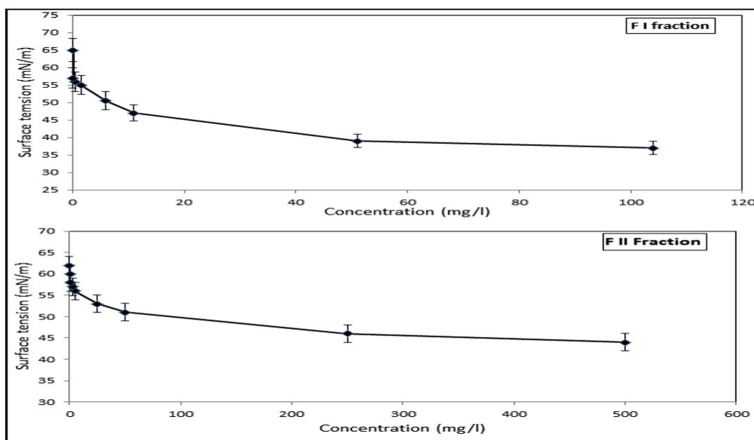
Figure 2: Critical micelle concentration (CMC) and minimum surface tension of the isolated SL fractions on the 12<sup>th</sup> day of fermentation (data were expressed as mean±S.E. of 4 experiments).
