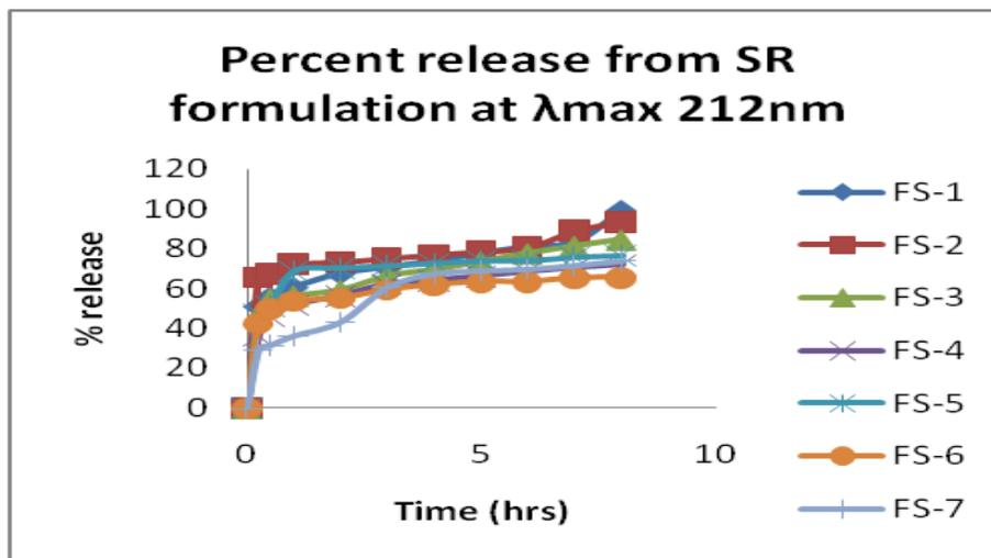
Figure 7: Percent release from SR formulation at  $\lambda_{max}$  212nm
