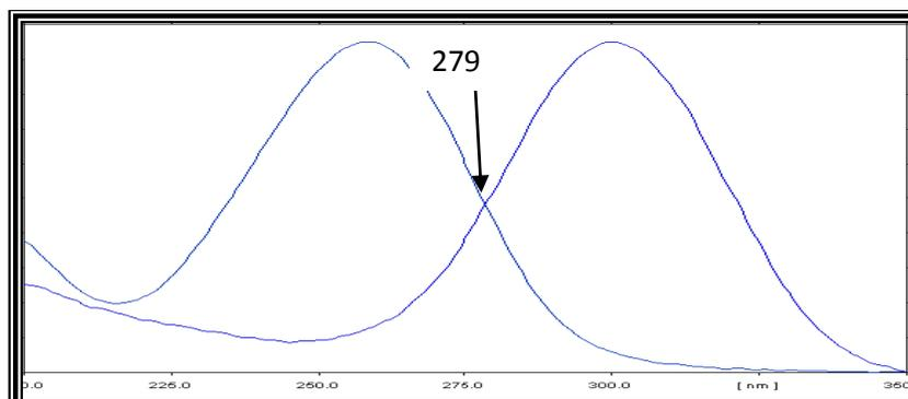
Figure 3: Overlaid absorption spectra for simultaneous estimation of BRZ and TM at 279
