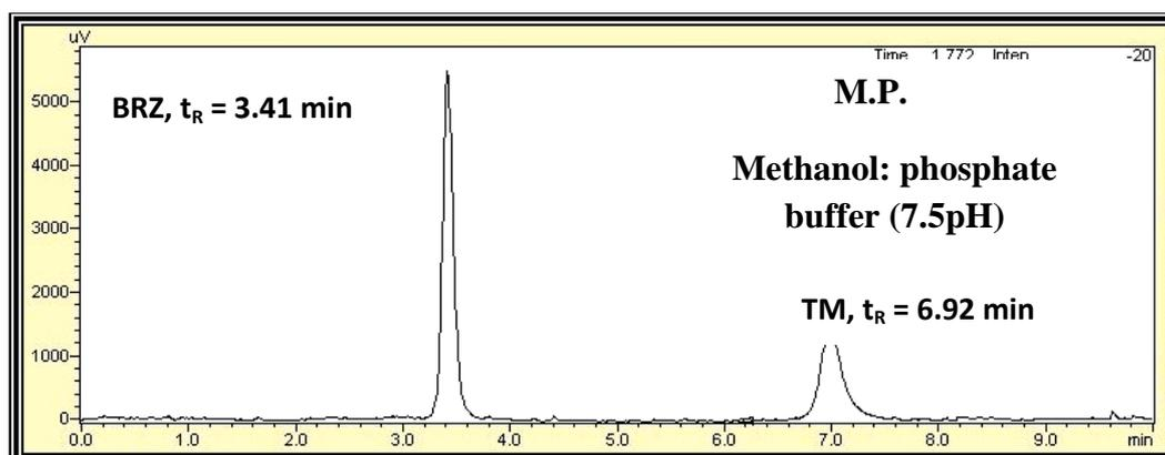
Figure 2: HPLC chromatogram under optimized conditions showing  $R_t = 3.41$  min for BRZ and  $R_t = 6.92$  min for TM
