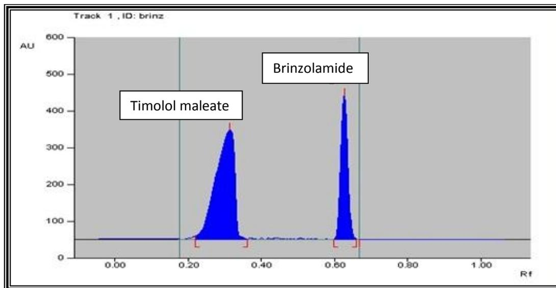
Figure 4: HPTLC densitogram under optimized conditions showing  $R_f = 0.35$  for TM and  $R_f = 0.64$  for BRZ
