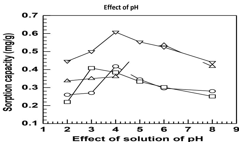
**Figure 1:** Effect of pH on the absorption capacity of metal ions by arenga pinata shell. on the condition of particle size  $\leq 150$  , concentration 50 mg / L , weight 1 g , volume 20 mL metal ion and flow rate of 2 mL / min . Note:: Cu<sup>+2</sup>(O), Pb<sup>+2</sup>(Δ), Ni<sup>+2</sup>(□), Co<sup>+2</sup>(▽)
