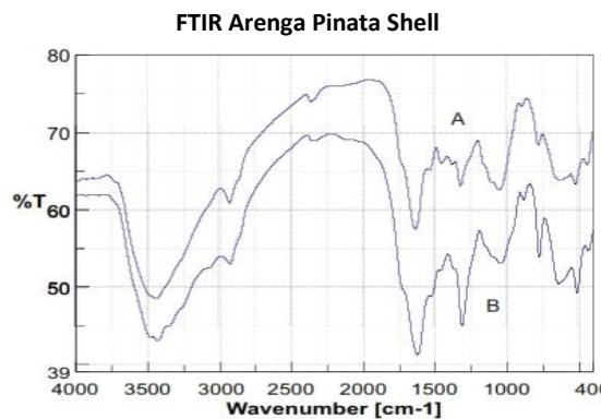
**Figure 9a.** FTIR arenga pinata shell. before (A) and after (B) uptake of metal ions Cu (II)
