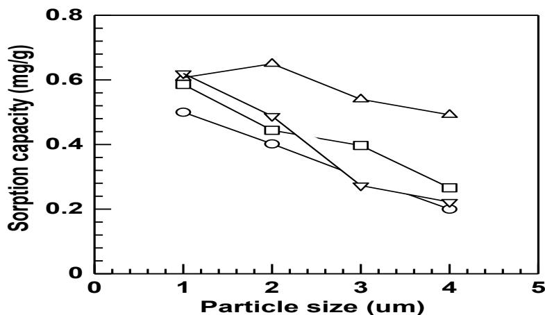
**Figure 2 . Effect of particle size of the arenga pinata shell. at optimum pH conditions , the concentration of 50 mg/L, weight 1 g, volume 20 mL metal ion and flow rate of 2 mL/min. Note : Cu<sup>+2</sup>(○), Pb<sup>+2</sup>(△), Ni<sup>+2</sup>(□), Co<sup>+2</sup>(▽) dan 1 ( $\leq 150 \mu\text{m}$ ), 2 (151-180  $\mu\text{m}$ ), 3 (181-250  $\mu\text{m}$ ), 4 (251-425  $\mu\text{m}$ )**
