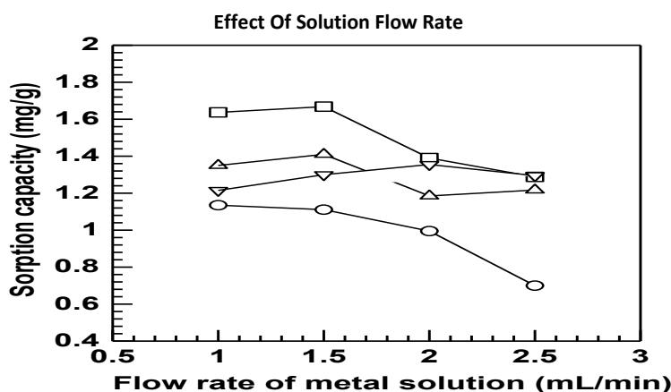
**Figure 5.** Effect of solution flow rate of the metal ion uptake capacity arenga pinata shell ( at the optimum pH, particle size ≤ 150, the concentration of 100 mg/L, 20 mL volume of the metal ion and a weight of 1 g. Note: Cu<sup>2+</sup>(○), Pb<sup>2+</sup>(△), Ni<sup>2+</sup>(□), Co<sup>2+</sup>(▽)
