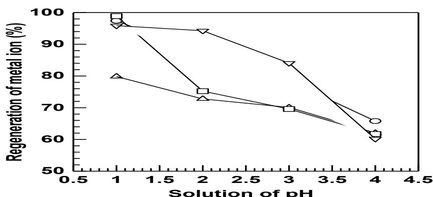
**Figure 8.** Effect of pH on the regeneration of the metal ion is absorbed by the arenga pinata shell. Note : Cu<sup>2+</sup>(○), Pb<sup>2+</sup>(△), Ni<sup>2+</sup>(□), Co<sup>2+</sup>(▽).
