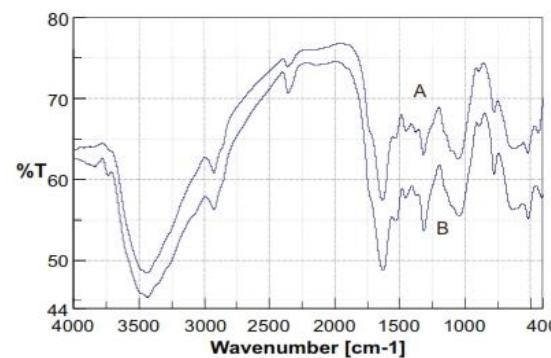
**Figure 9b.** FTIR arenga pinata shell. before (A) and after (B) uptake of metal ions Pb (II)
