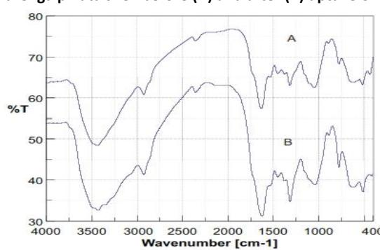
**Figure 9d.** FTIR arenga pinata shell before (A) and before (B) absorption of metal ions Co(II)
