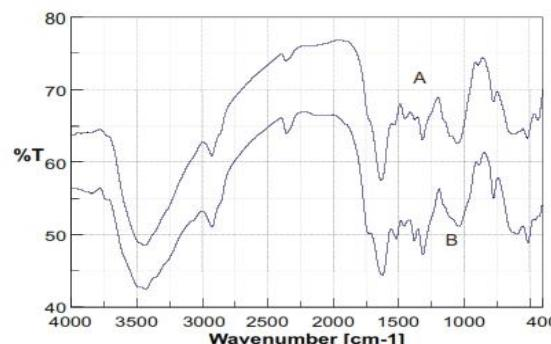
**Figure 9c.** FTIR arenga pinata shell before (A) and after (B) uptake of metal ions Ni (II)
