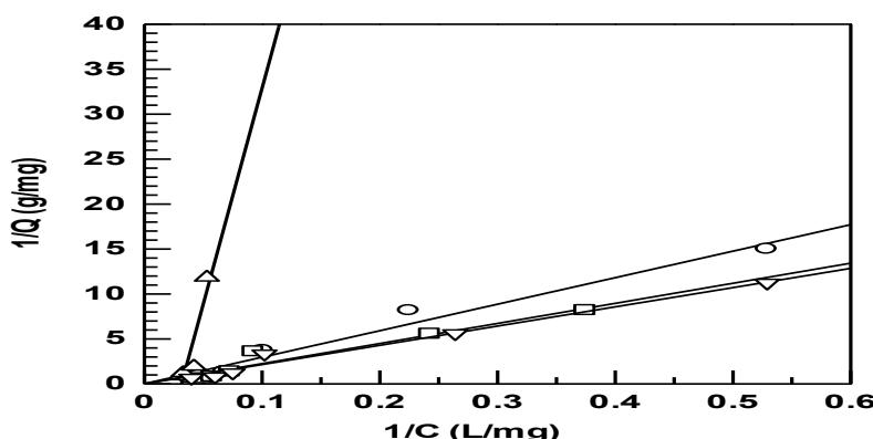
**Figure 4.** Langmuir isotherm of the metal ion is absorbed by the arenga pinata shell. Note : Cu<sup>+2</sup>(○), Pb<sup>+2</sup>(△), Ni<sup>+2</sup>(□), Co<sup>+2</sup>(▽)
