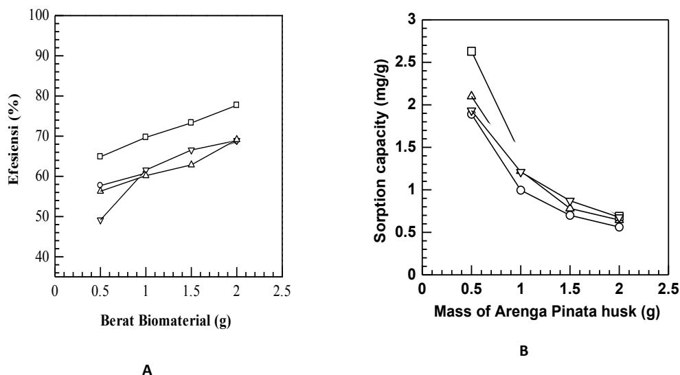
**Figure 6.** Heavy influence arenga pinata shell (A. Efficiency absorption, B. The absorption capacity) At optimum pH conditions, particle size  $\leq 150$ , the concentration of 100 mg/L, 20 mL volume of the metal ion and flow rate of 2 mL/min.
