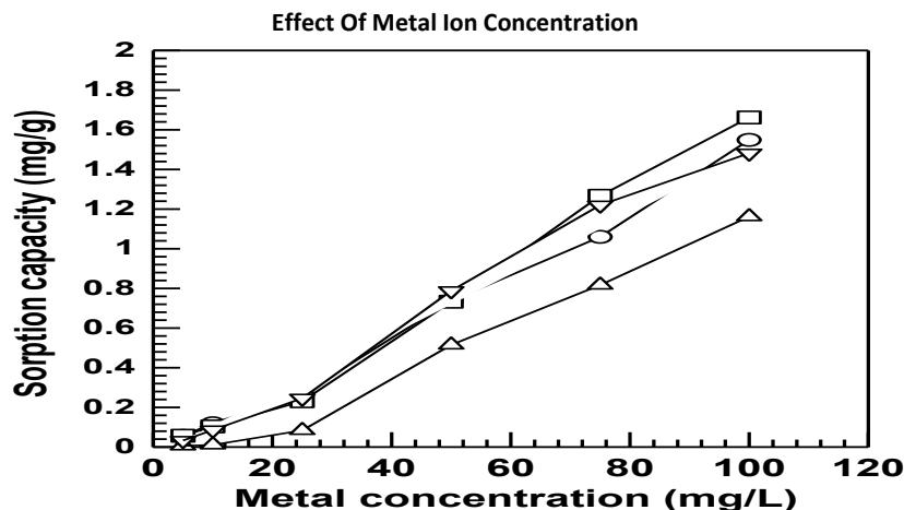
**Figure 3. Effect of metal ion concentration on the absorption capacity of the arenga pinata shell. at the optimum pH, particle size  $\leq 150$ , weighing 1 g, volume 20 mL metal ion and flow rate of 2 mL/sec. Note : Cu<sup>+2</sup>(○), Pb<sup>+2</sup>(△), Ni<sup>+2</sup>(□), Co<sup>+2</sup>(▽).**
