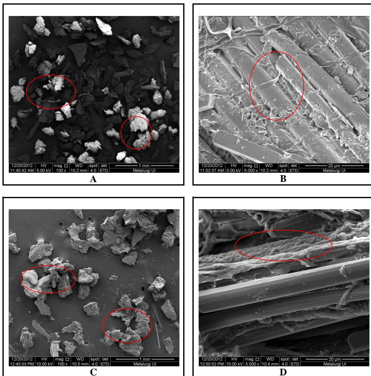
**Figure 10.** FE - SEM of the *Arenga pinnata* with 100X magnification (A), 5,000 X (B) and after absorption of metal ions Pb (II) 100 X (C) and 5000X (D)
