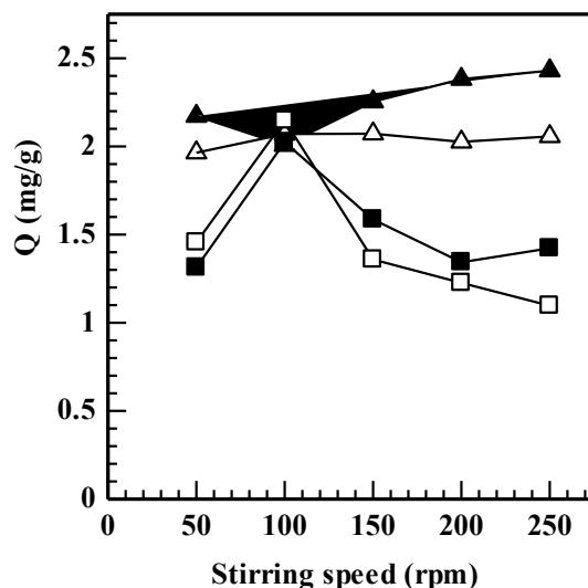
**Figure 3:** Effect of stirring speeds on the absorption of Pb (-■-), Cd (-□-), Cu (-Δ-), and Zn (-▲-); pH = 4; metal ions solution = 25 mL; concentration of solution = 10 mg/L; biomass weight = 0.1 g; contact time = 15 min.
