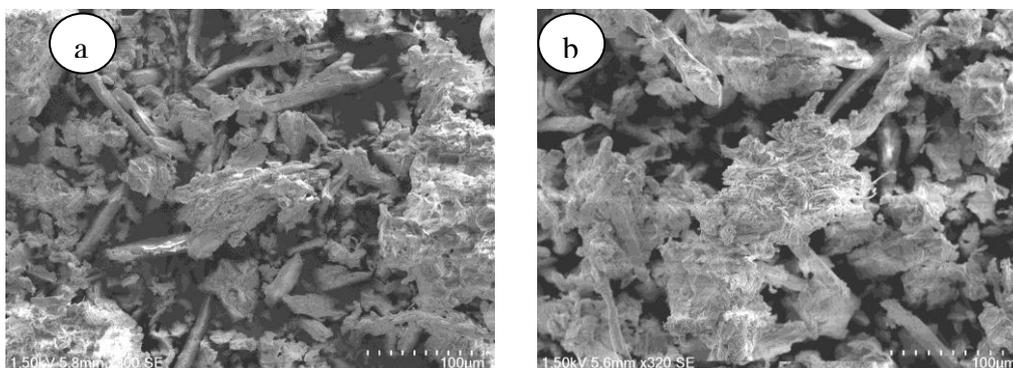
**Figure 8: SEM Results (a) before the biosorption (b) after the biosorption**
