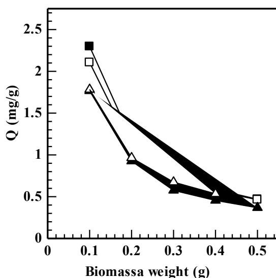
**Figure 4:** Effect of biomass weight on the absorption of Pb (-■-), Cd (-□-), Cu (-Δ-), and Zn (-▲-); pH = 4; metal ions solution = 25 mL; concentration of solution = 10 mg/L; stirring speed = 100 rpm; contact time = 15 min
