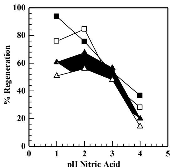
Figure 6: Regenerations of Pb (-■-), Cd (-□-), Cu (-Δ-), and Zn (-▲-); HNO<sub>3</sub> solution = 25 mL; biomass weight = 0.1 g; stirring speed = 100 rpm; contact time = 15 min.
