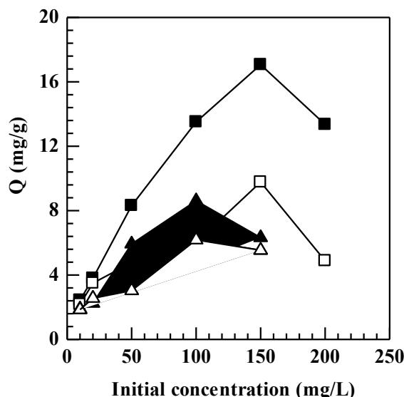
Figure 5: Effect of ion concentrations on the absorption of Pb (-■-), Cd (-□-), Cu (-Δ-), and Zn (-▲-), and Zn (II); pH = 4; metal ions solution = 25 mL; biomass weight = 0.1 g; stirring speed = 100 rpm; contact time = 15 min;
