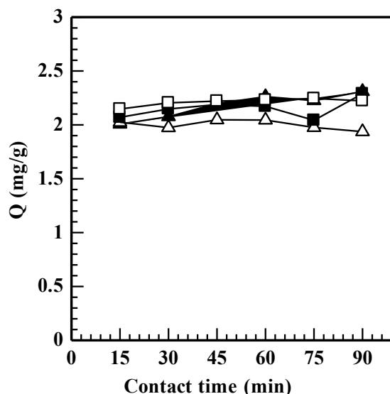
**Figure 2: Effect of time contacts on the absorption of Pb (■), Cd (□), Cu (Δ), and Zn (▲); pH = 4; metal ions solution = 25 mL; concentration of solution = 10 mg/L; biomass weight = 0.1 g; stirring speed = 100 rpm.**
