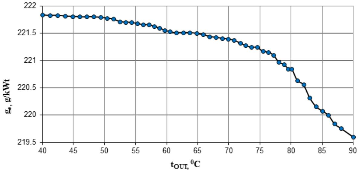
Figure 2: Dependence of specific fuel consumption on the CF temperature
