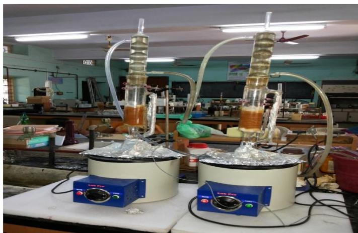
**Fig.2. Soxhlet apparatus for the M.Tinctoria roots extraction**
