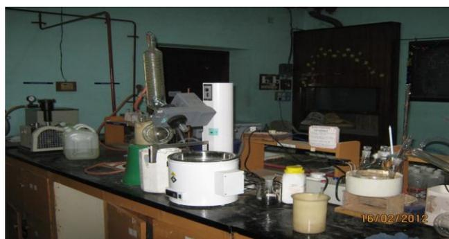
**Fig.3 Rotary Evaporator for Concentration**
