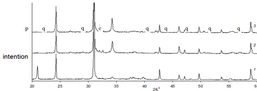
Figure 7: Diffractograms of the surface layer of concrete samples
