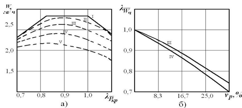
**Fig.9. Variation of operation estimations of VT-4S150DM tractor as a function of load rate  $\lambda_{P_{kp}}$  and coefficient of its variation  $v_p$  (I – 0%; II – 8.3%; III – 16.7%; IV – 25.0%; V – 33.3%): a)- hourly output  $\overline{W}_u$ ; b)-probability coefficient**
