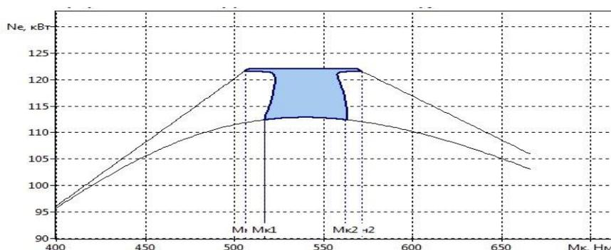
Fig.3. Optimum range for BF06M2012C engine.
