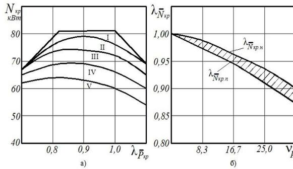
**Fig.8.** Variation of operation estimations of VT-4S150DM tractor as a function of load rate  $\lambda_{\overline{P}_{kp}}$  and coefficient of its variation  $v_p$  (I – 0%; II – 8,3%; III – 16,7%; IV – 25,0%; V – 33,3%): a)- haulage capacity  $\overline{N}_{kp}$  ; b)- probability coefficient
