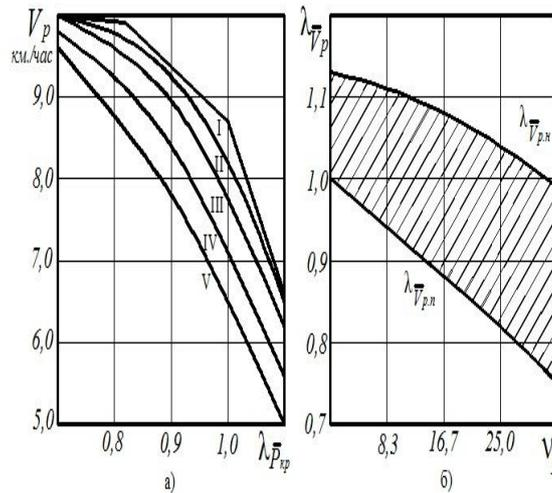
Fig.7. Variation of operation estimations of VT-4S150DM tractor as a function of load rate and coefficients of its variation  $v_p$  (I – 0%; II – 8.3%; III – 16.7%; IV – 25.0%; V – 33.3%): a)- traveling speed  $v_p$ ; b)- probability coefficient  $\lambda_{\bar{v}_p}$
