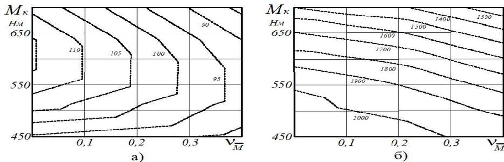
**Fig.1. 2D cross section of response surface characterizing alteration of effective power (a) and engine shaft RPM (b) as a function of torque and coefficient of variation.**
