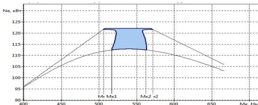
Fig.3. Optimum range for BF06M2012C engine.
