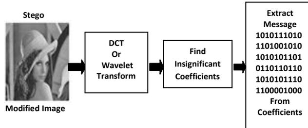
Figure: 6 Decoding block diagram
