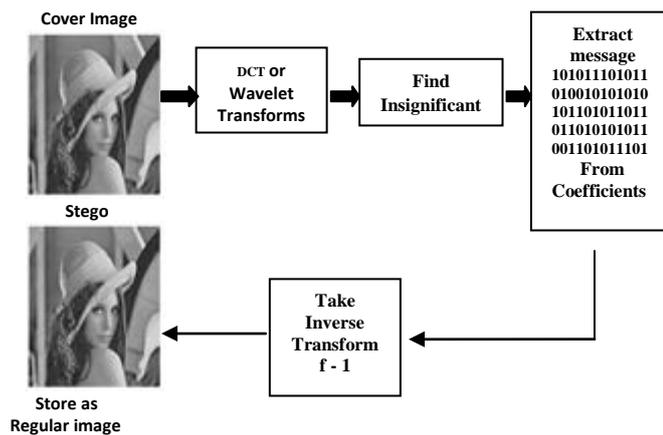
**Figure: 5 Encoding block diagram**
