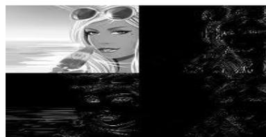
Figure: 4 2-Dimension wavelet transform applied through three transform levels
