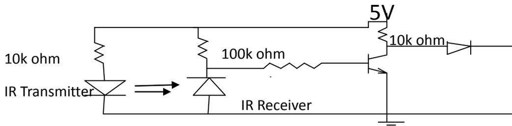
Figure 4: Heart Beat Monitoring IR Sensor module
