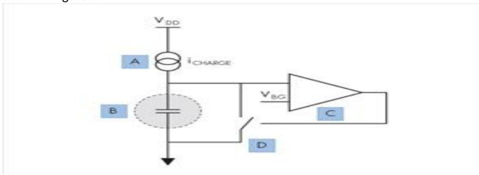
A - Current source; B - Sensor capacitor; C – Comparator; D - Discharge switch
