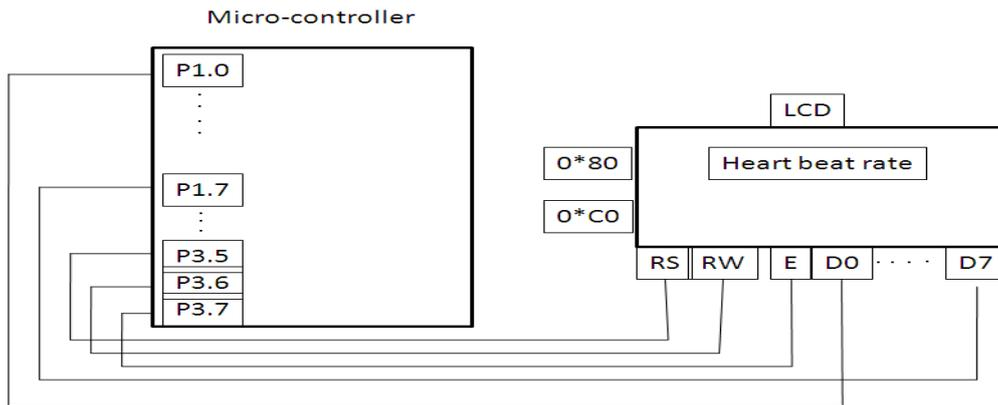
Figure 5: Interface circuitry for Heart beat rate display on LCD with Microcontroller
