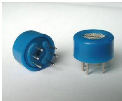
Figure : 5 MG811 sensor
