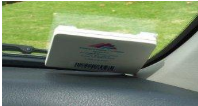
Figher4: RFID passive tag
