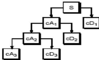
**Figure 3.3.3 (b)** Multilevel decomposition
