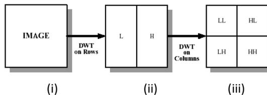
Figure: 3.3.1(C) DWT Block Diagram (i) Authentic Original Image (ii) Obtained Output image after the 1-D applied on Row input (iii) Output image after the second 1-D applied on row input
