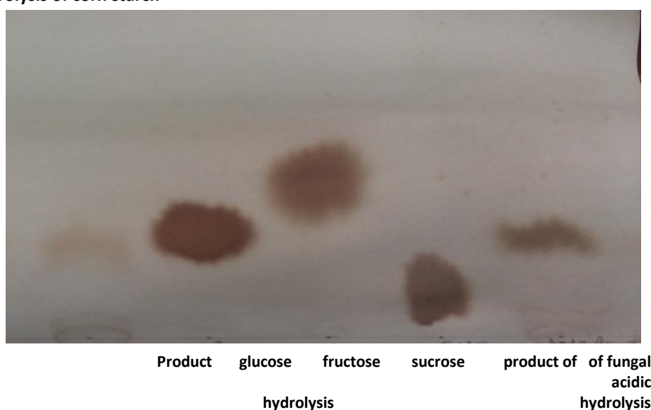
Figure 9: Product of fungal and acidic hydrolysis of corn starch
