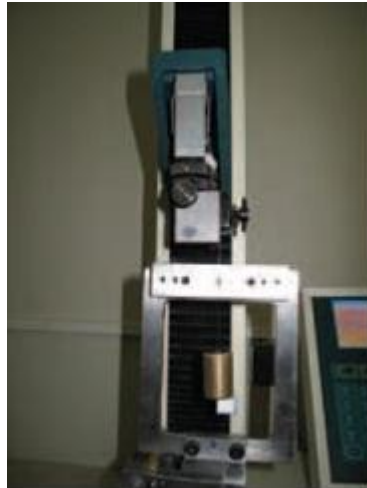
Figure 6: Friction measurements by means of a universal testing machine
