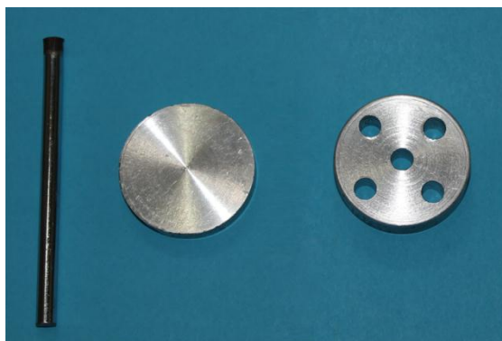
Figure 1: Metallic mould used for compressive strength testing
