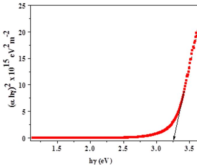
Figure 5: Optical band gap of mixed CdO and CeO<sub>2</sub> thin film
