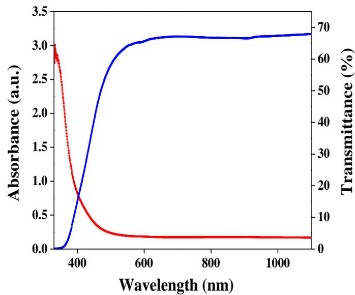
Figure 4: Optical absorption and transmission spectrum of mixed CdO and CeO<sub>2</sub> thin film
