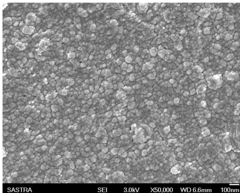
Figure 2: Scanning electron micrograph of mixed  $\text{CdO}$  and  $\text{CeO}_2$  thin film
