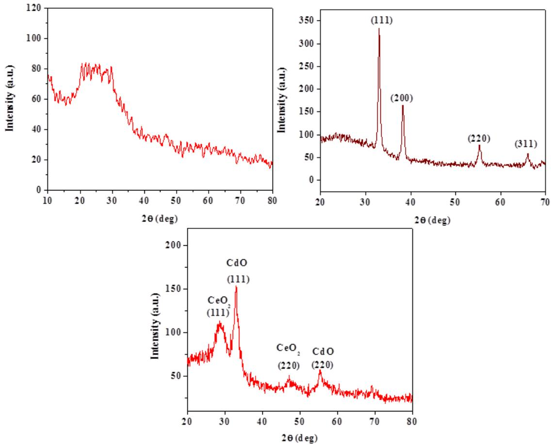
Figure 1(a) X- ray diffraction pattern for  $\text{CeO}_2$  thin film , (b)  $\text{CdO}$  thin film , (c) mixed  $\text{CdO}$  and  $\text{CeO}_2$  thin film.
