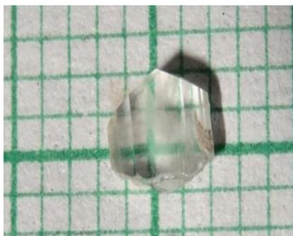
Figure 2: Photograph of as grown LASrT single crystal
