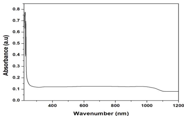
Figure 4: Optical absorption spectrum of LPT crystal
