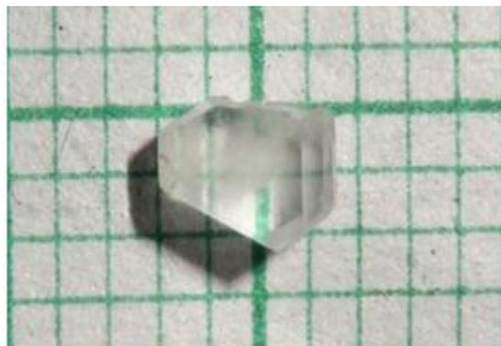
**Figure 2: Photograph of as grown LPT single crystal**
