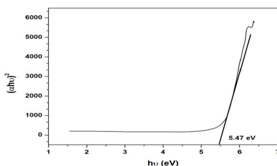
Figure 5 Optical band gap of LPT crystal
