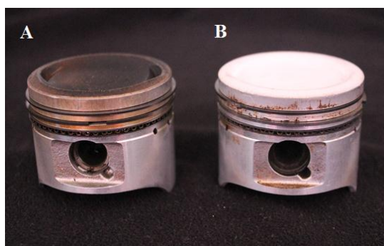
Figure 1: Uncoated Piston (A) and Piston coated with Alumina (B)
