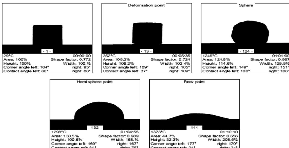
**Characteristic temperatures:** deformation temperature: 252 °C, deformation range: 252-1298 °C, sphere temperature: 1246 °C, hemisphere temperature: 1298 °C, flow range: 1298-1373 °C, flow temperature: 1373 °C (Figure 1).
