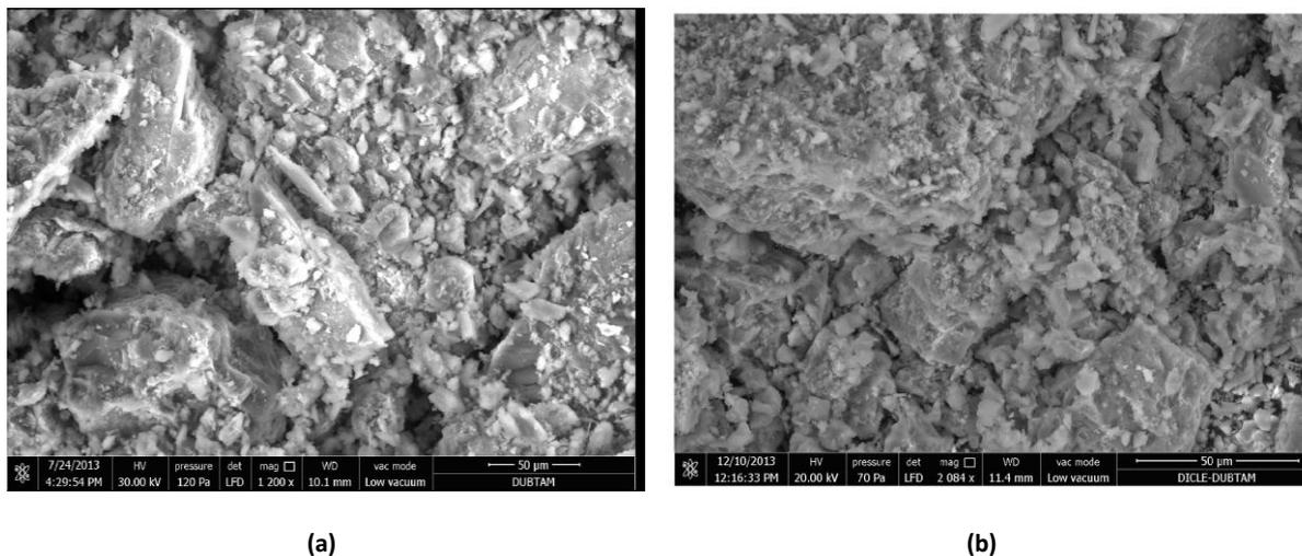
Figure 2: SEM micrographs for: (a) natural zeolite and (b) - Pb, Cu loaded zeolite.
