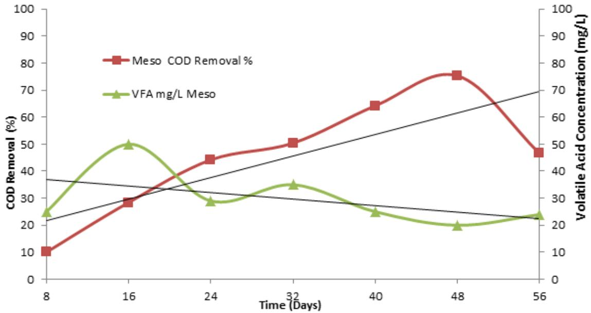
Figure 2: Variation in total volatile acids and COD removal profile during the mesophilic digestion
