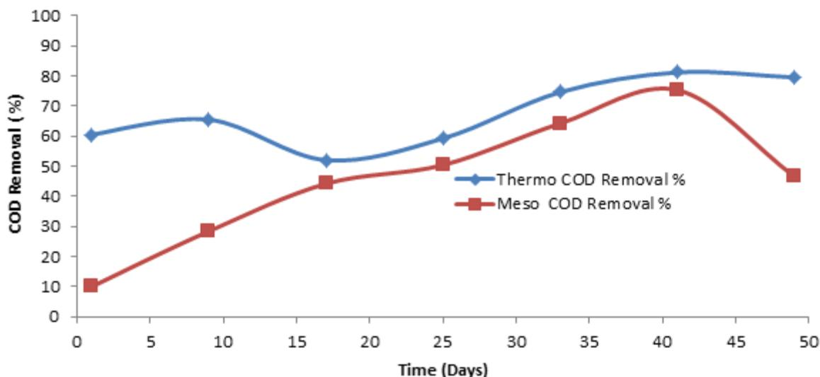
Figure 4: COD removal profile at mesophilic and thermophilic digestion
