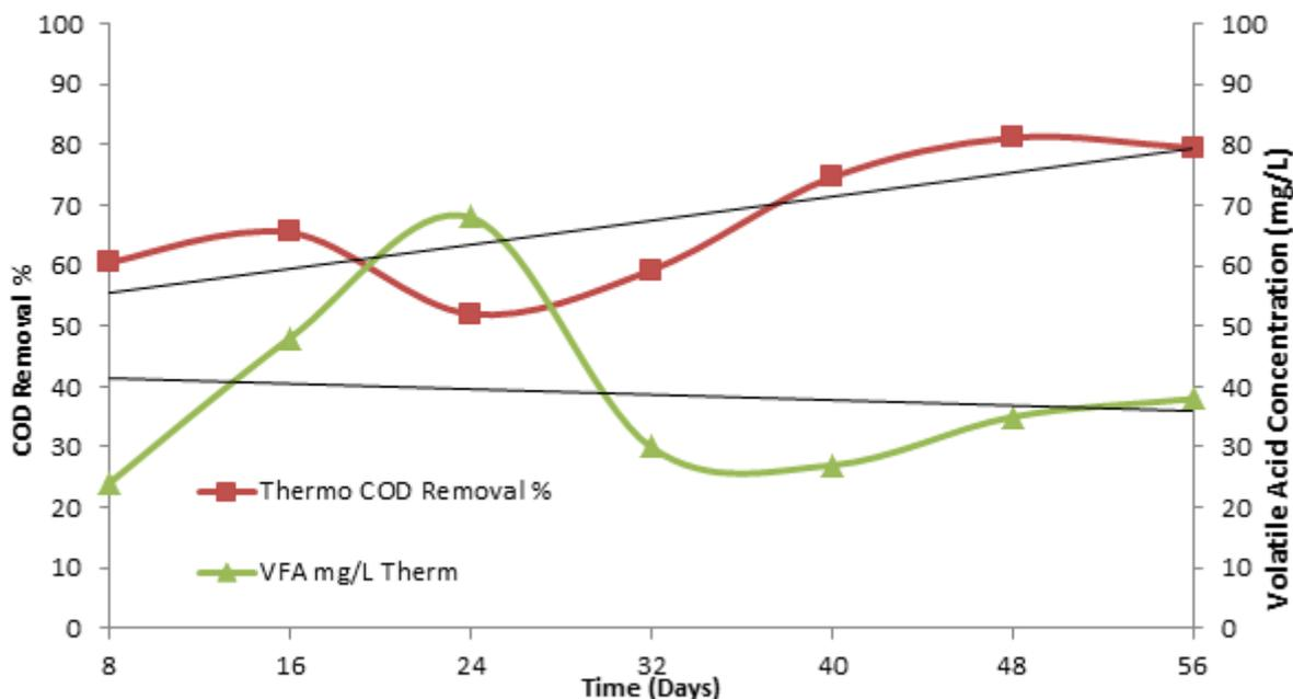
**Figure 1: Variation of total volatile acids and COD removal profile during thermophilic digestion**
