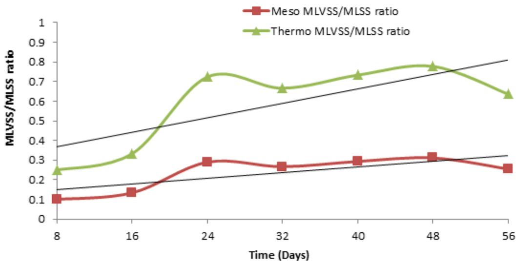
Figure 3: Comparison in variation of MLVSS/MLSS ratio in thermophilic and mesophilic digestion
