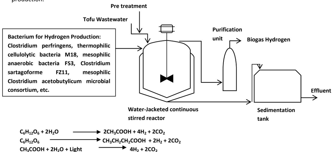
Figure 1. Schematic diagram for hydrogen production from tofu wastewater
