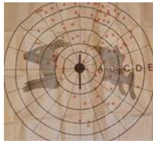
In the control firing from semi-automatic hunting rifles "MC 21-12", MP-153 and double-barreled shotguns IZH-27 with barrel lengths of 700mm without muzzle brakes-compensators and muzzle narrowing of 0.25 mm at a similar distance, the close grouping of pellets was at several times more up to 90 hits at a hundred-submultiple target using MC 21-12.
