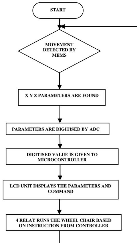
Figure 2: Flow chart for working of mems
