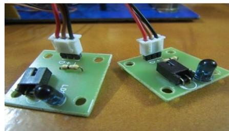
**Figure 16: Two IR sensors**
