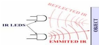
Figure 12: Object detection by IR sensor
