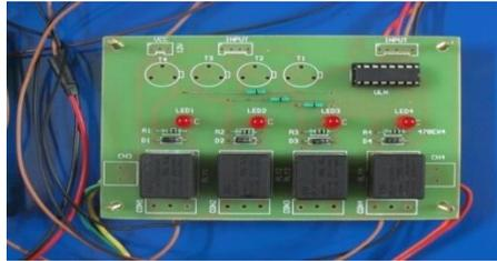
**Figure 20: Four relay board**
