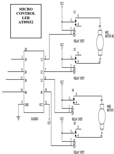
**Figure 6: Relay circuit diagram**
