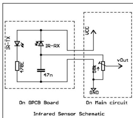
Figure 13: Circuit diagram of IR sensor
