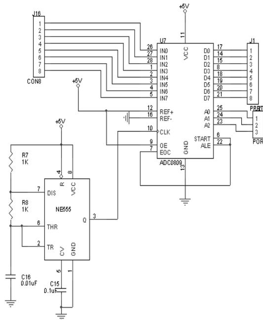
**Figure 5: ADC0809 circuit diagram**
