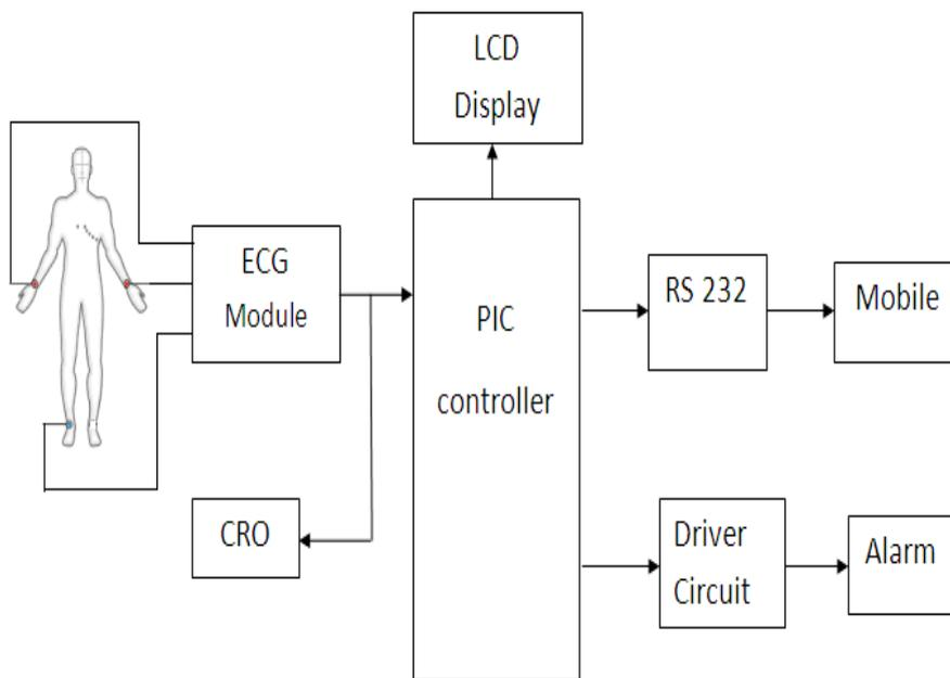
**Figure 2: Block Diagram**
