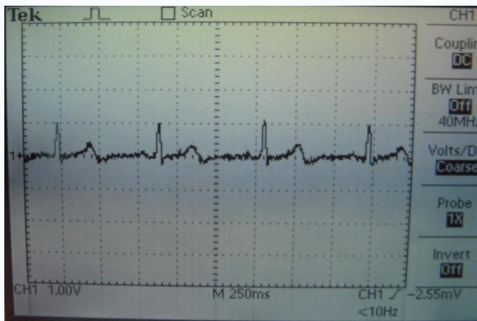
Figure 4: Normal signal displayed in CRO
