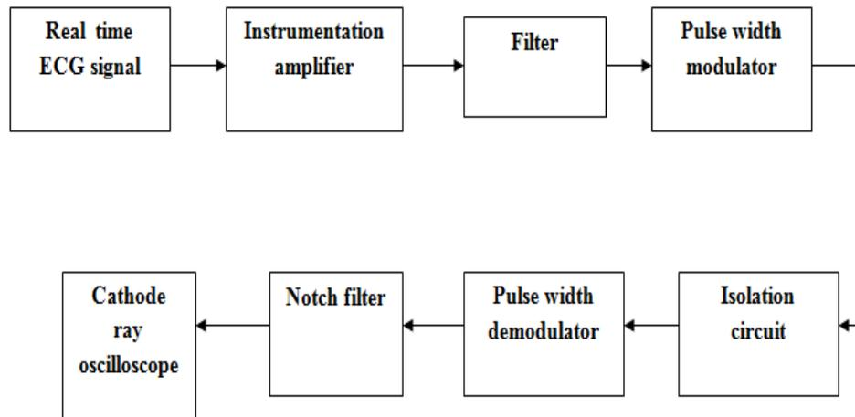
Figure 3: General block diagram of ECG hardware
