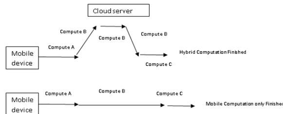
Figure 1: Computational offloading (Migration) process
