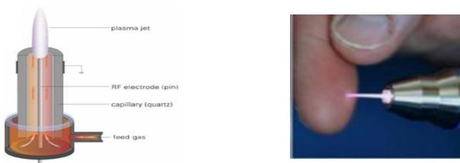
Figure 1: Schematic representation of a working model of a plasma apparatus.[8]
