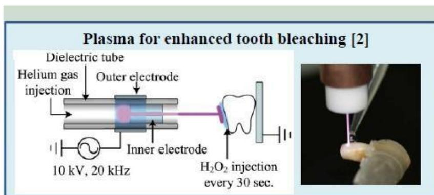
Figure 3: Schematic representation of a plasma apparatus for enhanced tooth bleaching [34].
