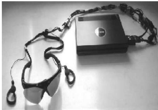
**Fig.4. "Seeing with sound" system (glasses With attached camera, ear speakers, and portable computer).**
