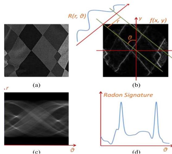
**Fig.3. (a) an intensity image of clothing pattern. (b) Radon transform performed on a maximum disk area within the gradient map (c) Result of Radon Transform. (d) Feature vector of Radon Signature.**
