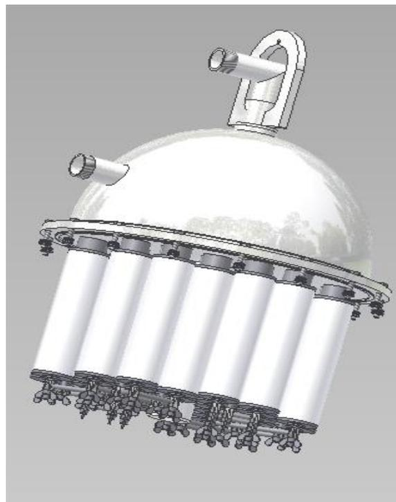
Figure 3: Cartridges of MSF-5.0 membrane module
