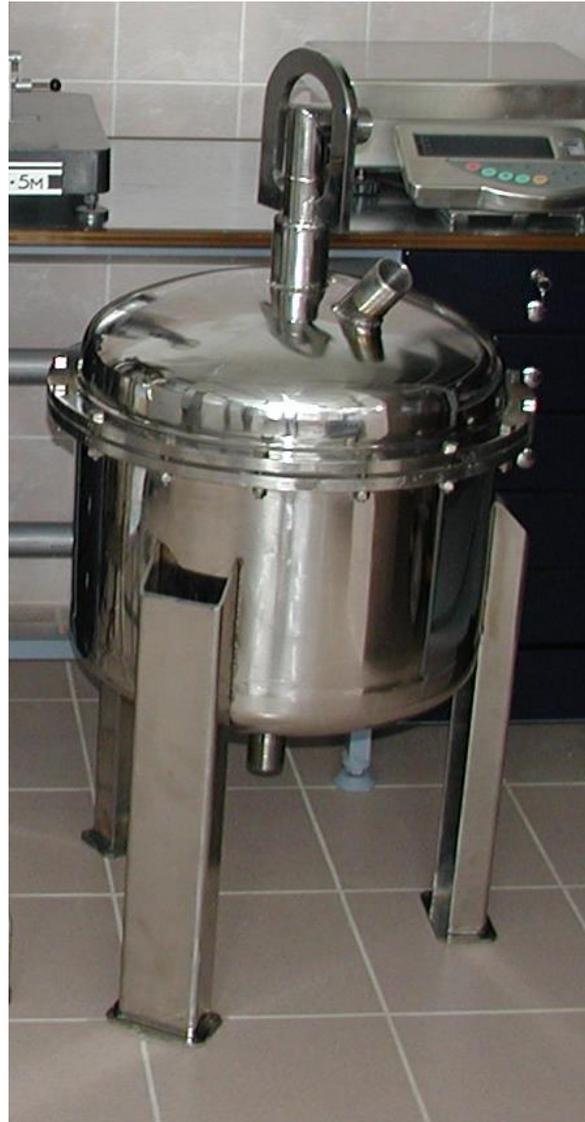
**Figure 4: MSF-5.0 membrane module**
