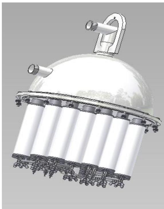
Figure 3: Cartridges of MSF-5.0 membrane module
