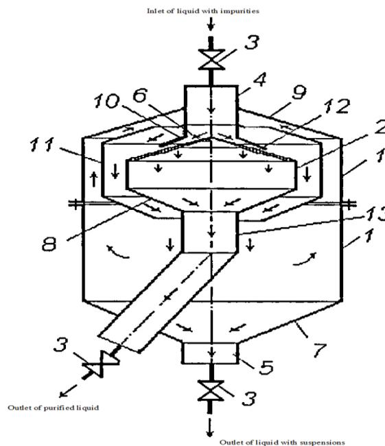
**Figure 1: Module for preliminary purification of liquids**
