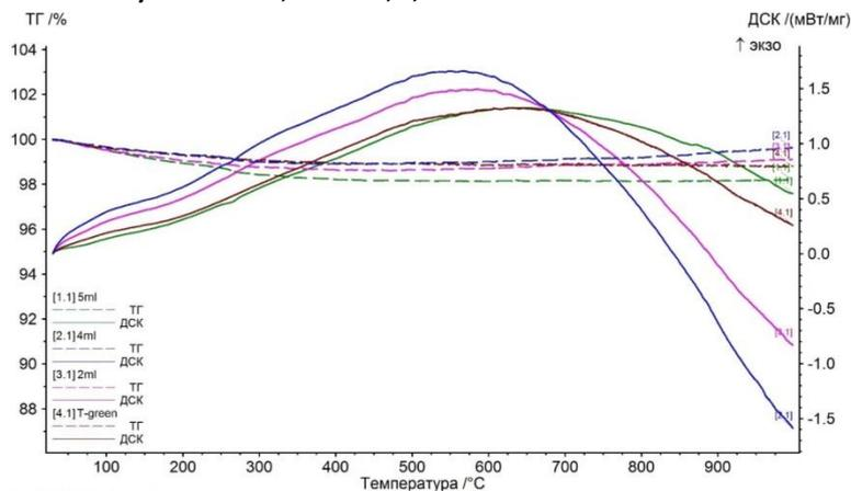
Figure 7: The results of thermal analysis of the mixtures of CW and zinc oxide. The curves of differential thermal analysis: 1.1 – 3%; 2.1 – 9%; 3,1 – 12% . 4.1 – source CW.
