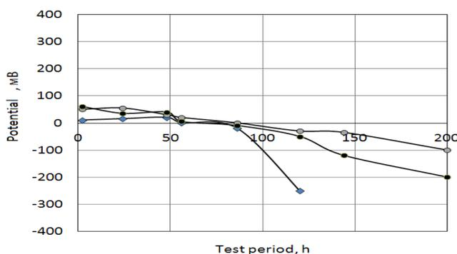
**Figure 2: Kinetics of corrosive potential of aqueous extracts**
