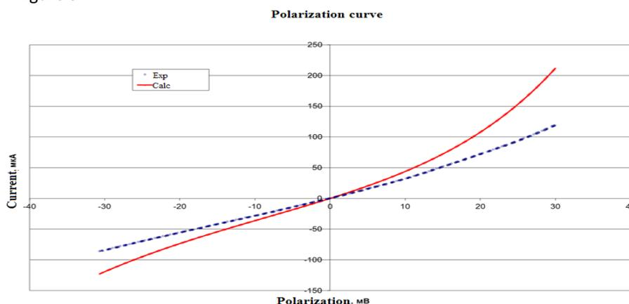
Figure 3: Potentiodynamic polarization curves, characterizing steel behavior 08 kp in contact with extract of CW
