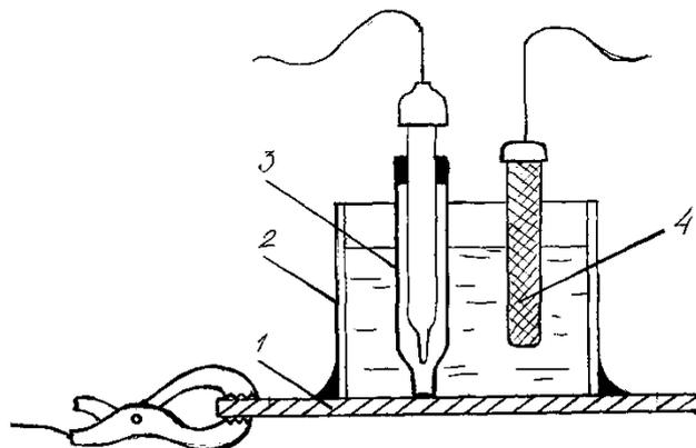
1 – steel plate; 2 – glass cylinder; 3 – silver-chlorine electrode; 4 – auxiliary electrode
