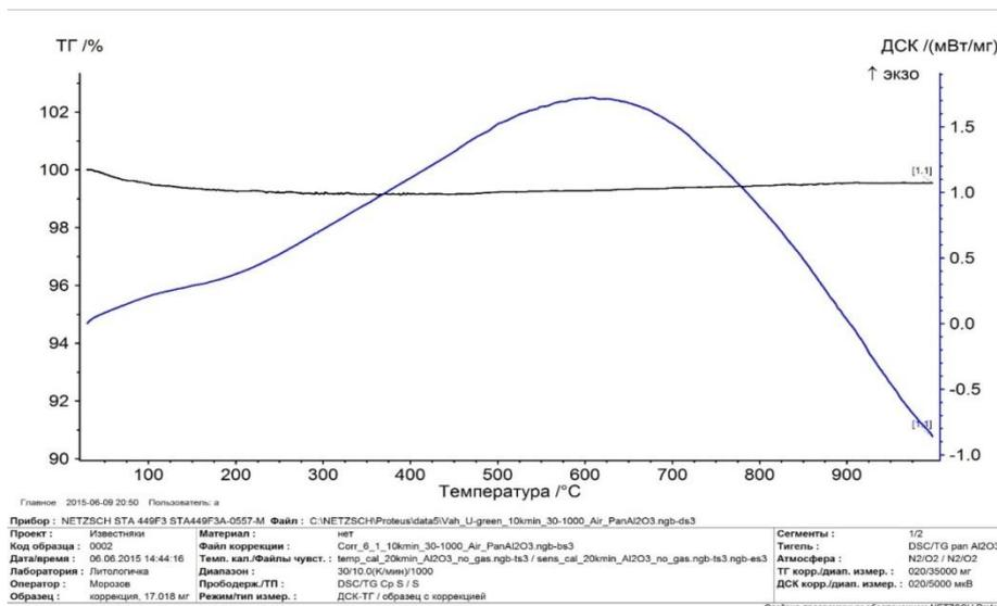
**Figure 5: The results of thermoanalysis of CW. 1 – the curve of differential thermoanalysis, 2 – the curve of thermogravimetry.**
