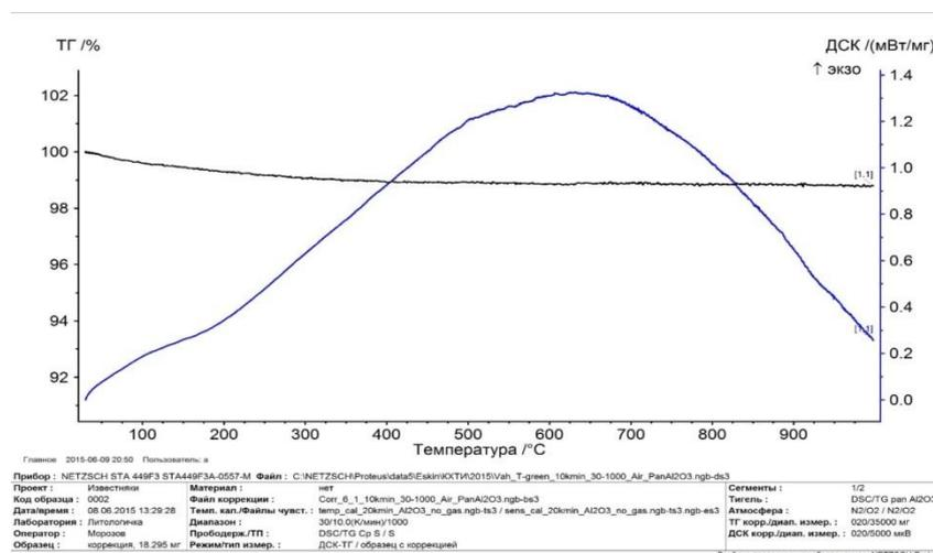
Figure 4: The results of thermoanalysis of FW. 1 – the curve of differential thermoanalysis, 2 – the curve of thermogravimetry,
