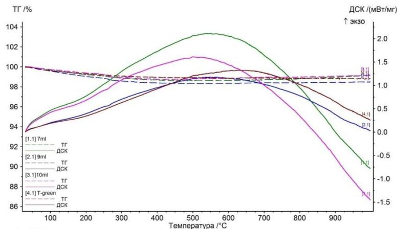
Figure 6: The results of thermoanalysis of mixtures of FW and zinc oxide. The curves of differential thermal analysis: 1.1 – 3%; 2.1 – 9%; 3,1 – 12%. 4.1 – source FW.
