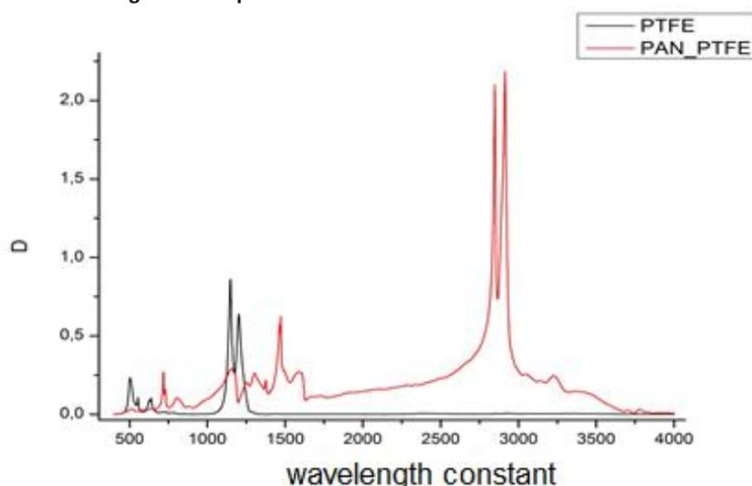
Figure 3: IR absorption spectra of PTFE: lower - PTFE top - membrane PTFE-PANI [7]
