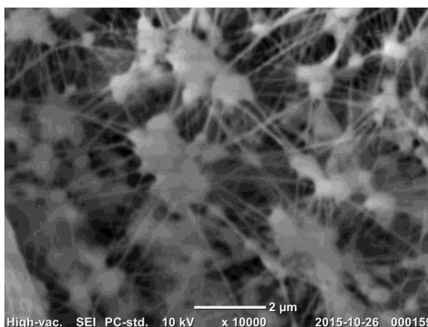
**Figure 1: Snapshot of the original PTFE membrane.**
