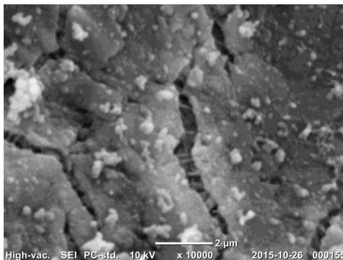
Figure 2: The picture is a modified PTFE membrane-PANI.
