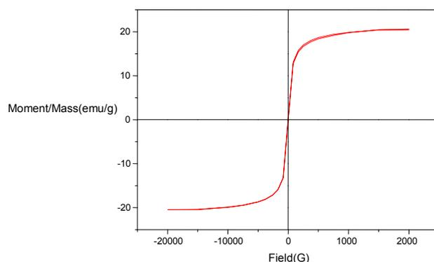
Fig (5): hysteresis curve of starch  $\text{Fe}_3\text{O}_4$ .
