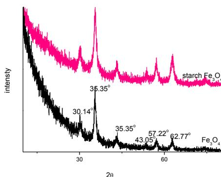
Fig (4): the XRD patterns of pure  $\text{Fe}_3\text{O}_4$ , starch  $\text{Fe}_3\text{O}_4$ .
