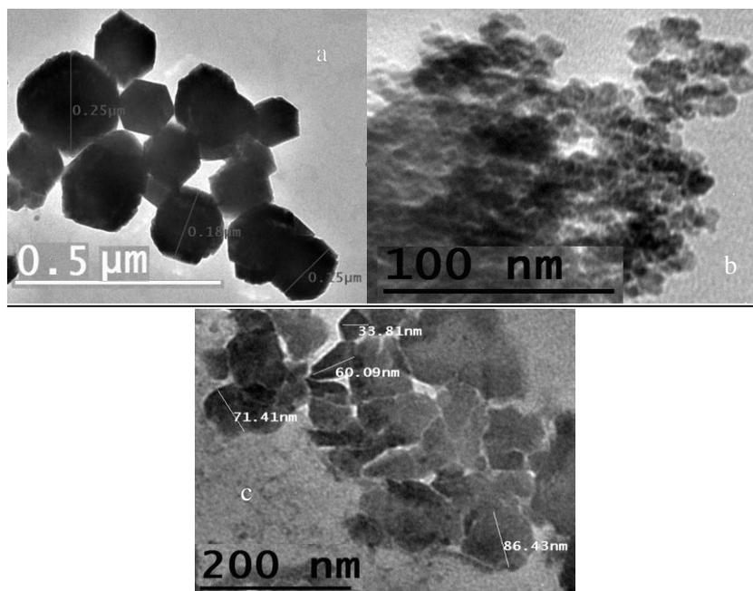
Fig (3): TEM images of stained native starch (a), unstained starch  $\text{Fe}_3\text{O}_4$  (b) and stained starch  $\text{Fe}_3\text{O}_4$ (c).
