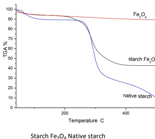
**Fig (2): the TGA curve for native starch, starch Fe<sub>3</sub>O<sub>4</sub> nanoparticles and pure Fe<sub>3</sub>O<sub>4</sub>.**
