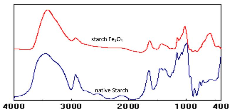
Fig (1): FTIR spectra of native starch and starch  $Fe_3O_4$  nanoparticle
