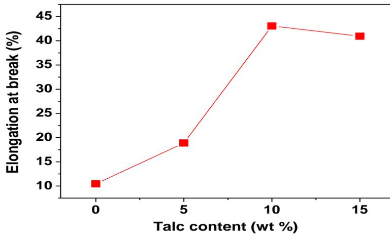
Figure 2: Elongation at break variations of polystyrene/talc composites as function of talc content.
