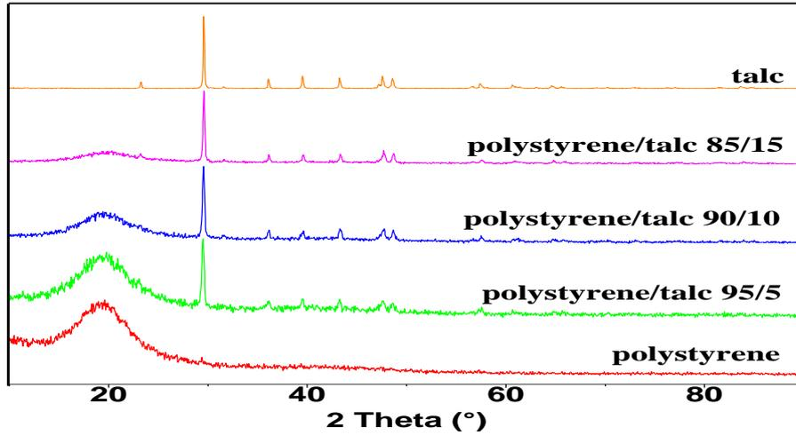
Figure 1: XRD patterns of polystyrene, talc and polystyrene/talc composites.
