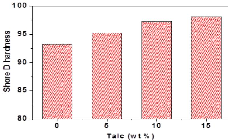
Figure 4: Shore D hardness changes of polystyrene composites as function of talc loading
