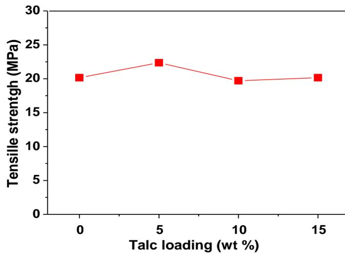
Figure 3: Tensile strength variations of polystyrene/talc composites as function of talc loading.
