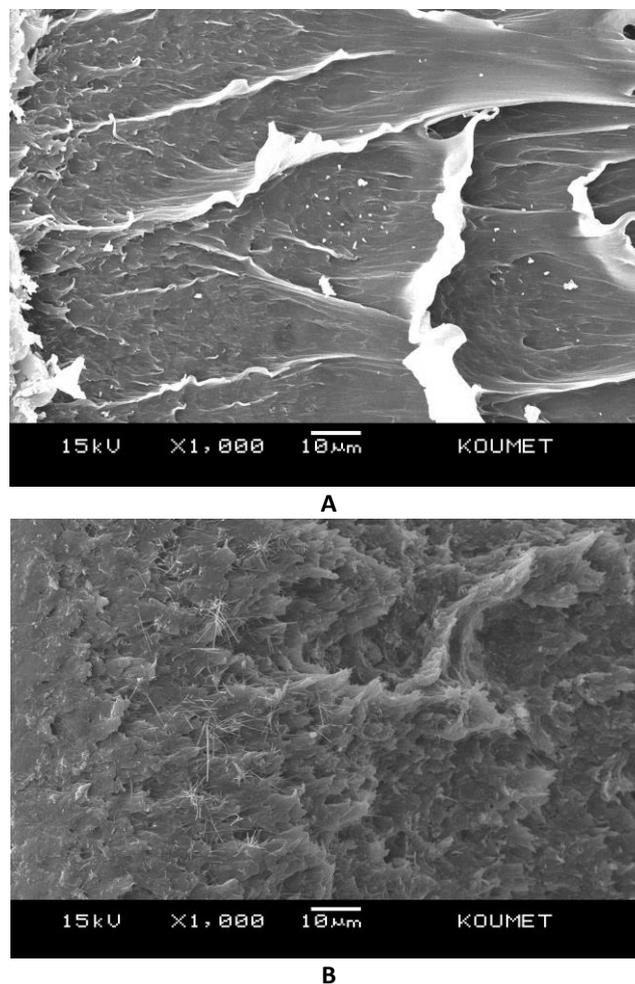
Figure 6: SEM micrographs; (A) polystyrene reinforced 5% of talc, (B) polystyrene reinforced 10% of talc.
