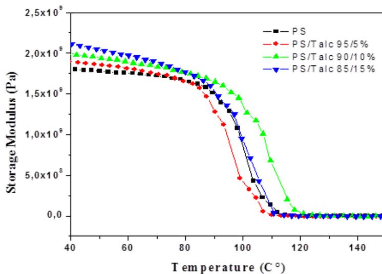
Figure 5: Storage modulus of neat PS and PS/talc composites as a function of temperature
