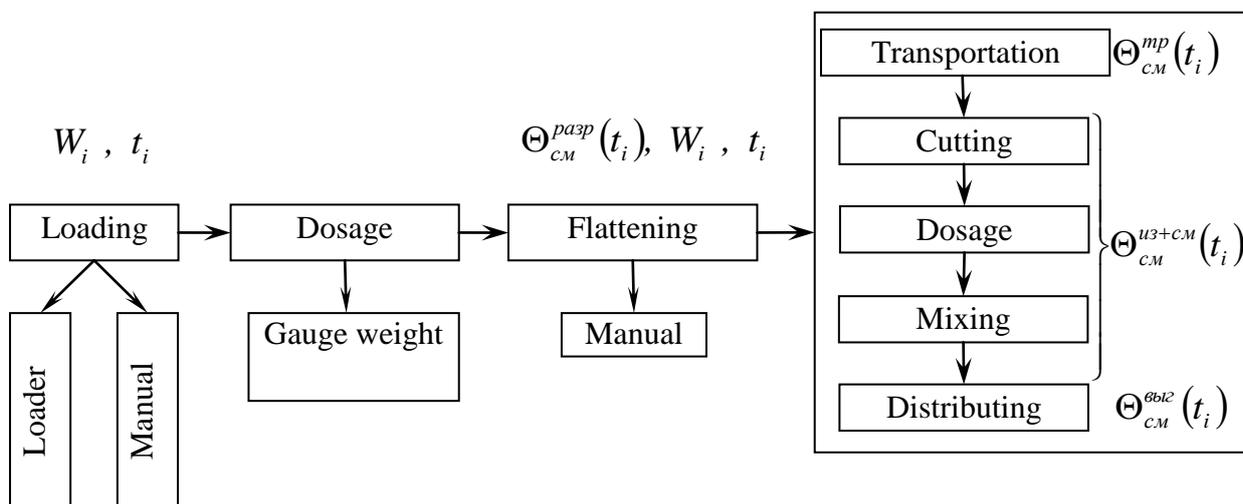
Figure 2: Structural and technological scheme of the line of distribution of fodder mixtures at small farms.
